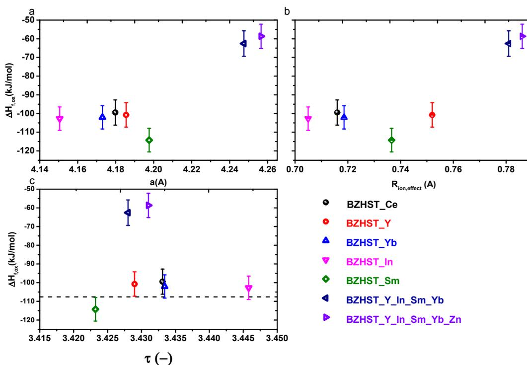
**Figure 3** Enthalpies of drop solution formation from the oxides at 25 °C as a function of unit cell parameter (a), average ionic radius of B-cation (b), and extended Goldschmidt factor<sup>35</sup> (c), ionic radii according to Shannon.<sup>36</sup> The experimental uncertainties are indicated.
