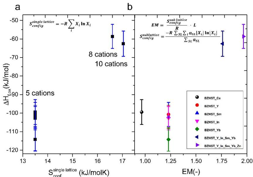
**Figure 2** Enthalpies of drop solution formation from the oxides at 25 °C as a function of configurational entropy for a single lattice model ( $S_{\text{conf}}^{\text{single lattice}}$ ) and entropy metrics (EM) based on the sublattice model ( $S_{\text{conf}}^{\text{sublattice}}$ ). The experimental uncertainties are indicated.
