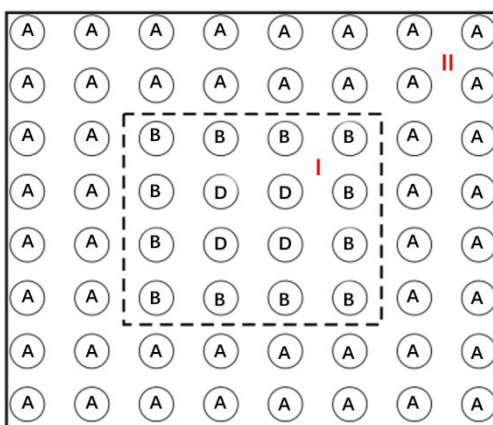
Figure 1: The division diagram of region I and region II in the multiscale approach. The atoms marked with 'D' indicate internal DFT atoms or core atoms with defects. Atoms marked with 'A' denote external MD atoms. Atoms marked with 'B' indicate boundary atoms.
