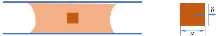
Figure 1. Growth of a cubic crystal of a in width in a liquid solution. The thickness of diffusion layer is \delta .
