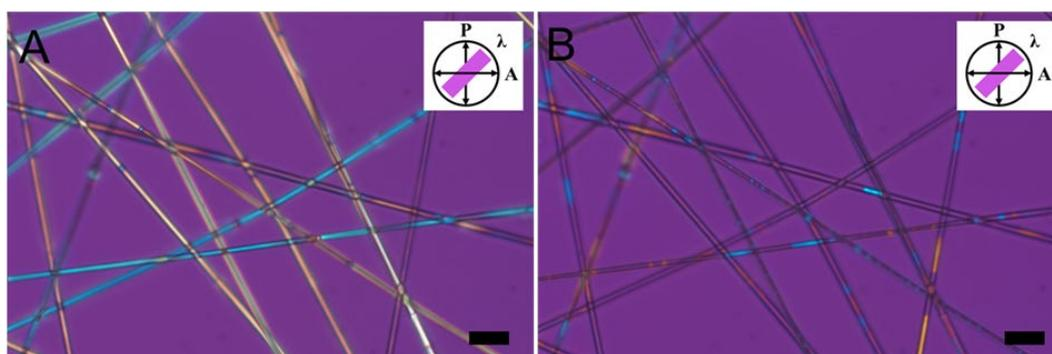
Figure 8. Crossed POM images with a quarter-wave retardation plate of fibers with 1.5 wt%  $C_4AzoC_6PEG_3$  at 25 °C before (A) and after (B) UV irradiation. Scale bars = 10  $\mu m$ .
