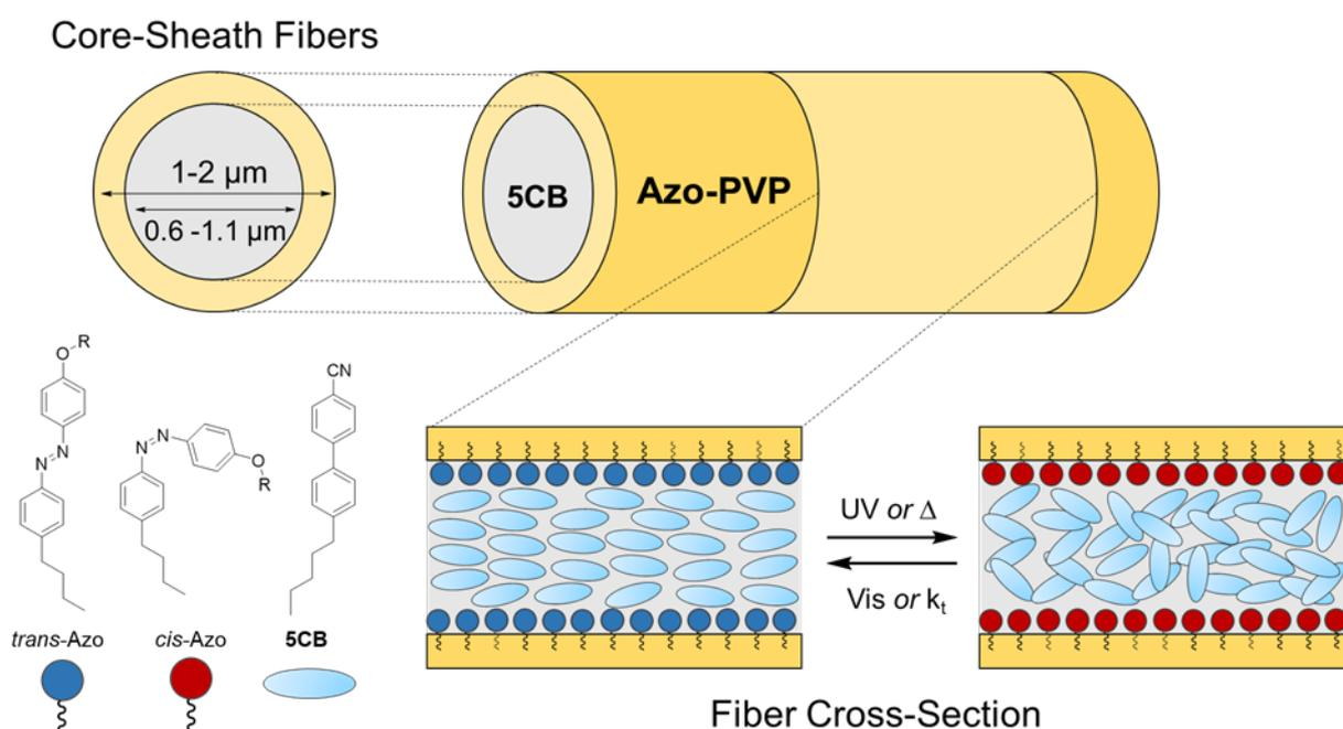
Scheme 1. An overview of the work presented in this system. Electrospun nanofibers are prepared with a PVP sheath doped with 0–3 wt% of an azobenzene-based surfactant and a neat 5CB core. Irradiation of the nanofibers containing  $C_4AzoC_6PEG_3$  results in the disorder of the LC core and a depression of the  $N \rightarrow I$  transition temperature which is reversible with visible light.
