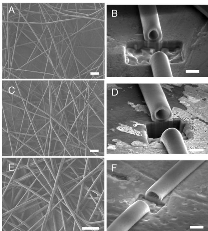
**Figure 4.** SEM images of nanofibers made with 0 wt% (A, B), 1.5 wt% (C, D), and 3 wt% (E, F) of  $C_4AzoC_6PEG_3$ . FIB-SEM images showing milled out sections of the fibers revealing the core-sheath morphology. Scale Bars: A, C, E = 10  $\mu m$ ; B, D, F = 1  $\mu m$ .
