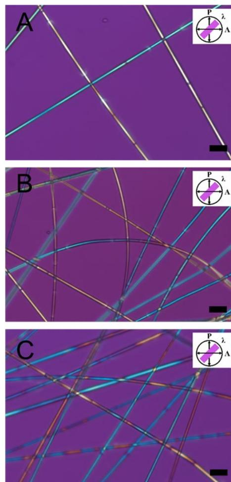
**Figure 7.** POM images of electrospun fibers viewed with a quarter-wave retardation plate. A. 0.0 wt%  $C_4AzoC_6PEG_3$ , B. 1.5 wt%  $C_4AzoC_6PEG_3$ , C. 3.0 wt%  $C_4AzoC_6PEG_3$ .
