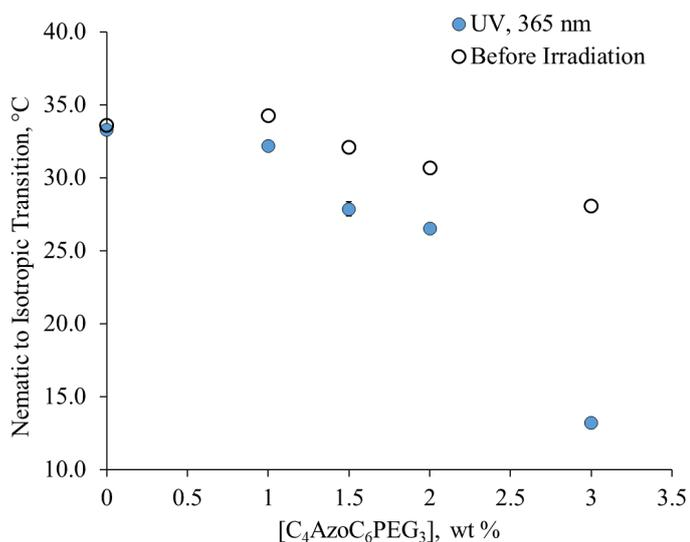
**Figure 3.**  $T_{N \rightarrow I}$  of coaxial electrospun fibers containing a **5CB** core and a PVP sheath with 0-3 wt% of **C<sub>4</sub>AzoC<sub>6</sub>PEG<sub>3</sub>**. The phase transitions were identified by the loss of birefringence of the LC core and error bars are the result of triplicate measurements. The transition temperatures were measured before (as spun) and after UV irradiation at 365 nm for 5 seconds.
