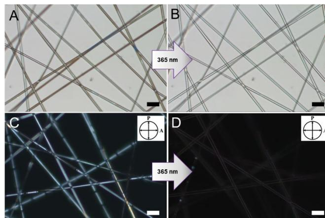
**Figure 5.** POM images of 1.5 wt%  $C_4AzoC_6PEG_3$  at 25 $^{\circ}C$  before (A, C) and after (B, D) UV irradiation. Images A and B were taken using polarized light illumination and images C and D were taken under crossed polarizers. Scale bars = 10  $\mu m$ .
