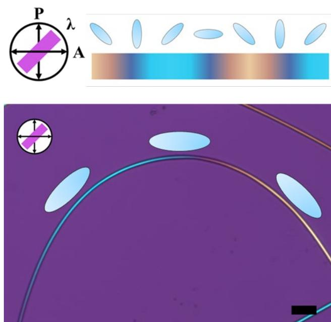
**Figure 6.** Electrospun nanofiber with 1.0 wt%  $C_4AzoC_6PEG_3$  and a **5CB** core viewed with crossed POM and quarter-wave retardation plate showing axial planar alignment of the LC within the fiber. Color bar at top depicts how the image color corresponds to the LC orientation. Color change along the fiber indicates that the LCs are aligned along the fiber long axis. Scale bar = 10  $\mu m$ .
