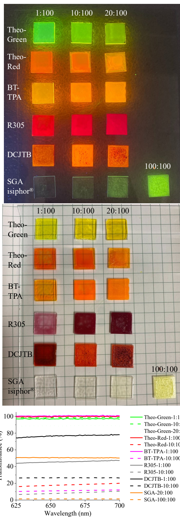
Fig. 8. Comparison of light converting efficacy (top) and transparency (middle) of inorganic phosphors and organic dyes. Blending ratio (converter:SBS) are also labelled. (bottom) transmittance of the light-converting films.
