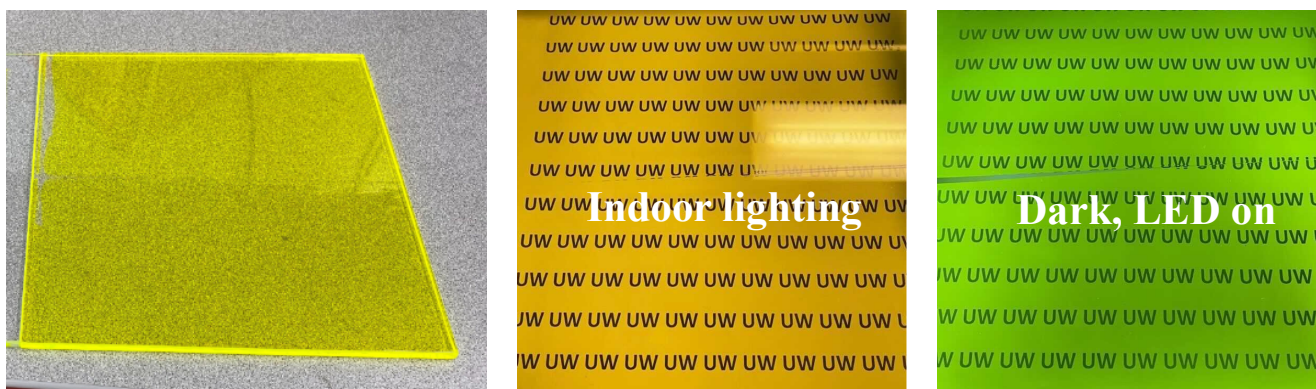
Fig. 9. (left) as-fabricated waveguide by blade-coating the Theo-Green-SBS composite on a glass substrate; (middle & right) demonstration of transparency and non-glare feature of the edge-lit lighting device based on the waveguide shown on the left.
