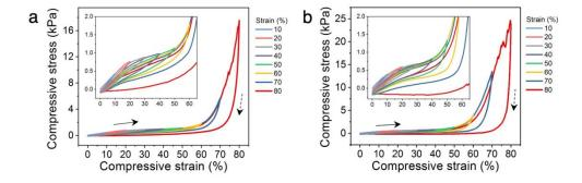
**Figure 5.** Cyclic compression behavior of PANI hydrogels. Stress-strain curves during loading-unloading to various strains for (a) Kelvin lattice with 14% relative density, and (b) octet lattice with 16% relative density. Arrows and dashed arrows represent the loading and unloading directions, respectively. A loading and unloading rate of 100% min<sup>-1</sup> was used.
