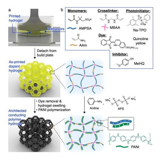
**Figure 1.** (a) Schematic diagram illustrating the printing and synthesis of architected PANI hydrogels. (b) Chemical structures for the components in the aqueous precursor solution.
