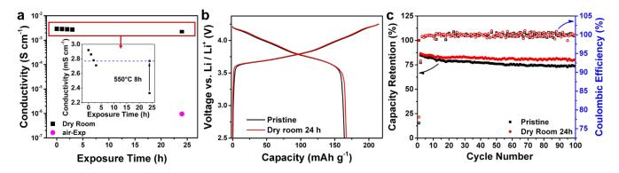
**Figure 6.** a) Ionic conductivity of pristine LPSCl, LPSCl samples exposed in a dry room for 1, 2, 3, 24 hours, a heat-treated sample following 24 hours of dry room exposure, and air-exposed LPSCl. b) 1<sup>st</sup> cycle voltage profiles, c) capacity retention and Coulombic efficiency of NCM811 | LPSCl | LiIn cells assembled using pristine or 24h dry room exposed LPSCl electrolytes.
