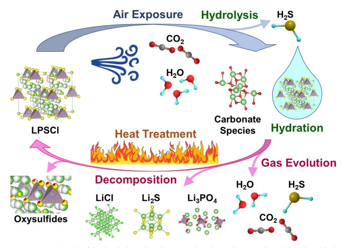
Figure 1. Schematic of the chemical reactions that occur when  $Li_6PS_5Cl$  is exposed to ambient air and during the subsequent heat treatment process.
