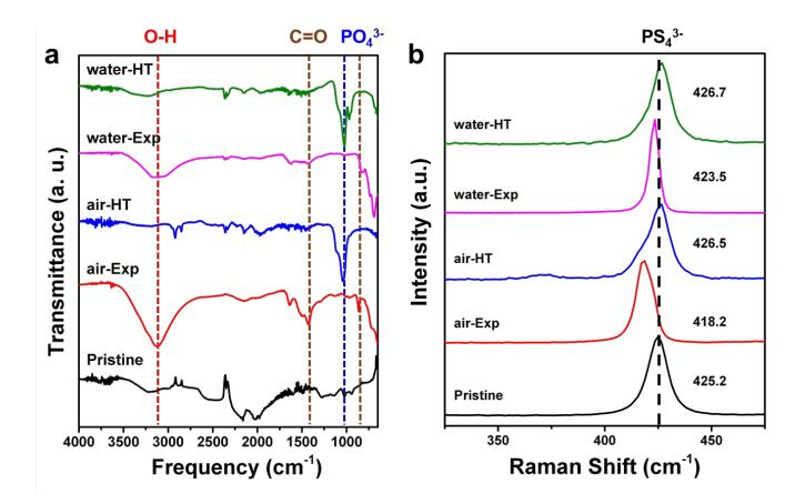
**Figure 3.** a) FTIR and b) Raman spectra of the pristine, exposed and heat-treated LPSCl samples. The main peaks of interested are represented by dashed lines on the FTIR spectra, while the Raman spectra only shows the  $PS_4^{3-}$  peak.
