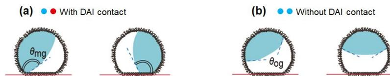
**Fig. 7.** Possible mechanism of the PSI edge pinned at the DAI after the DAI contact. Differences in the contact angle according to the position of the gelatin-rich domain (glue) (a) with and (b) without DAI contact.
