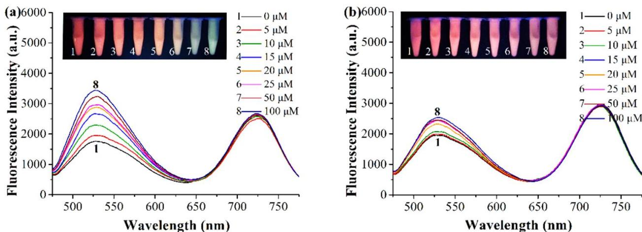
**Figure 5.** Fluorescence response of 2,4-D-MIPs (a) and the NIPs counterpart (b) with increasing concentration of 2,4-D from 0 to 100  $\mu\text{M}$ . Reprinted and adapted with permission from Hou, Y.; Zou, Y.; Zhou, Y.; Zhang, H. Biological Sample-Compatible Ratiometric Fluorescent Molecularly Imprinted Polymer Microspheres by RAFT Coupling Chemistry. *Langmuir* 2020, 36 (41), 12403–12413. Copyright 2020 American Chemical Society.
