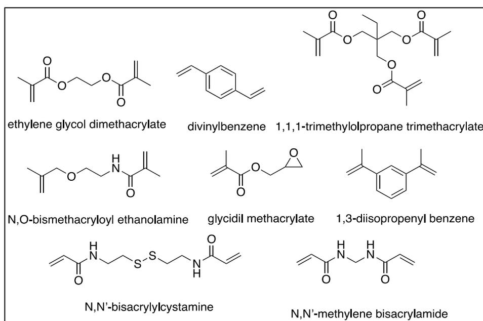
Figure 3. Common crosslinkers utilized in the synthesis of MIPs.
