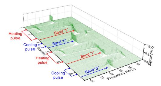
**Fig. 3.** Evolution of resonance frequency and amplitude of the  $MoS_2$  resonator with time during the heating and cooling cycles, which can be used to program the resonator into different frequency bands.
