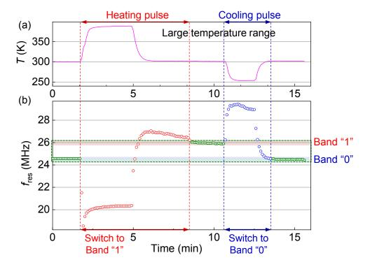
**Fig. 4.** (a) Temperature profile and (b) the corresponding evolution of device resonance frequency, for 1 heating-cooling pulse cycle with data extracted from the resonance spectra in Fig. 3, showing the process of using the heating (red data points) and cooling pulses (blue data points) to program the resonator into frequency band "1" and band "0", respectively (green data points). The heating and cooling pulse temperatures are 116°C and -20°C, respectively.
