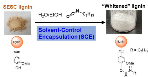
Fig. 1 Reaction route of whitening lignin derivatives via reaction with organic isocyanates in accordance with SCE. Typical photographs are (left) neat SESC lignin powder and (right) hexyl modified SESC lignin described as “whitened” lignin. The reaction route of lignin and isocyanate represents an example of a possible general process, not specific, selective reaction, i.e. , other hydroxy groups in lignin derivative can also react with the isocyanate group.
