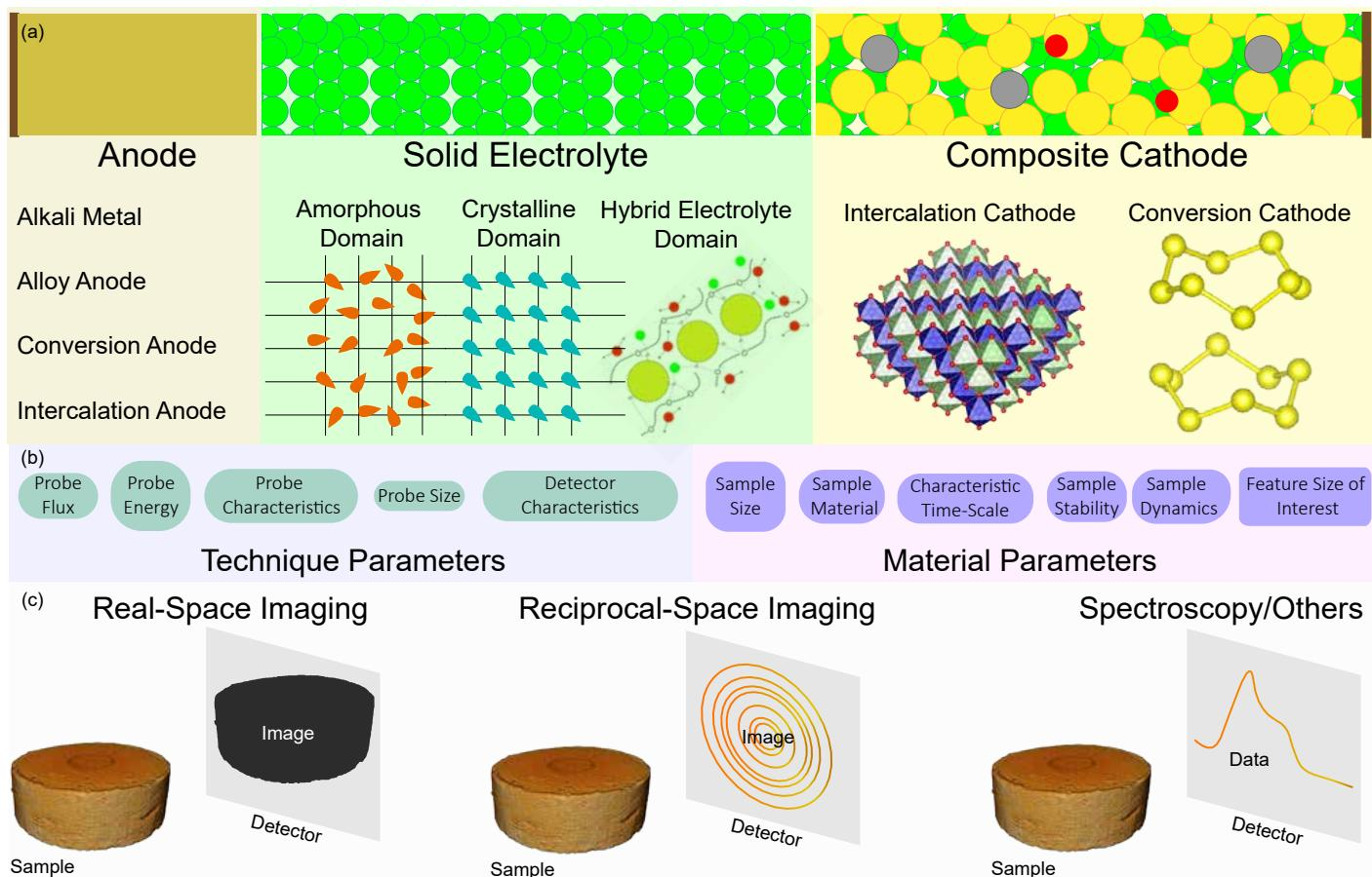
**Fig. 3** Overview of characterization techniques to study SSBs. (a) Schematic diagram showing material types for different components of the solid state battery. (b) Sample and technique parameters that influence measurement. (c) Schematic illustrating non-destructive SSB characterization techniques.
