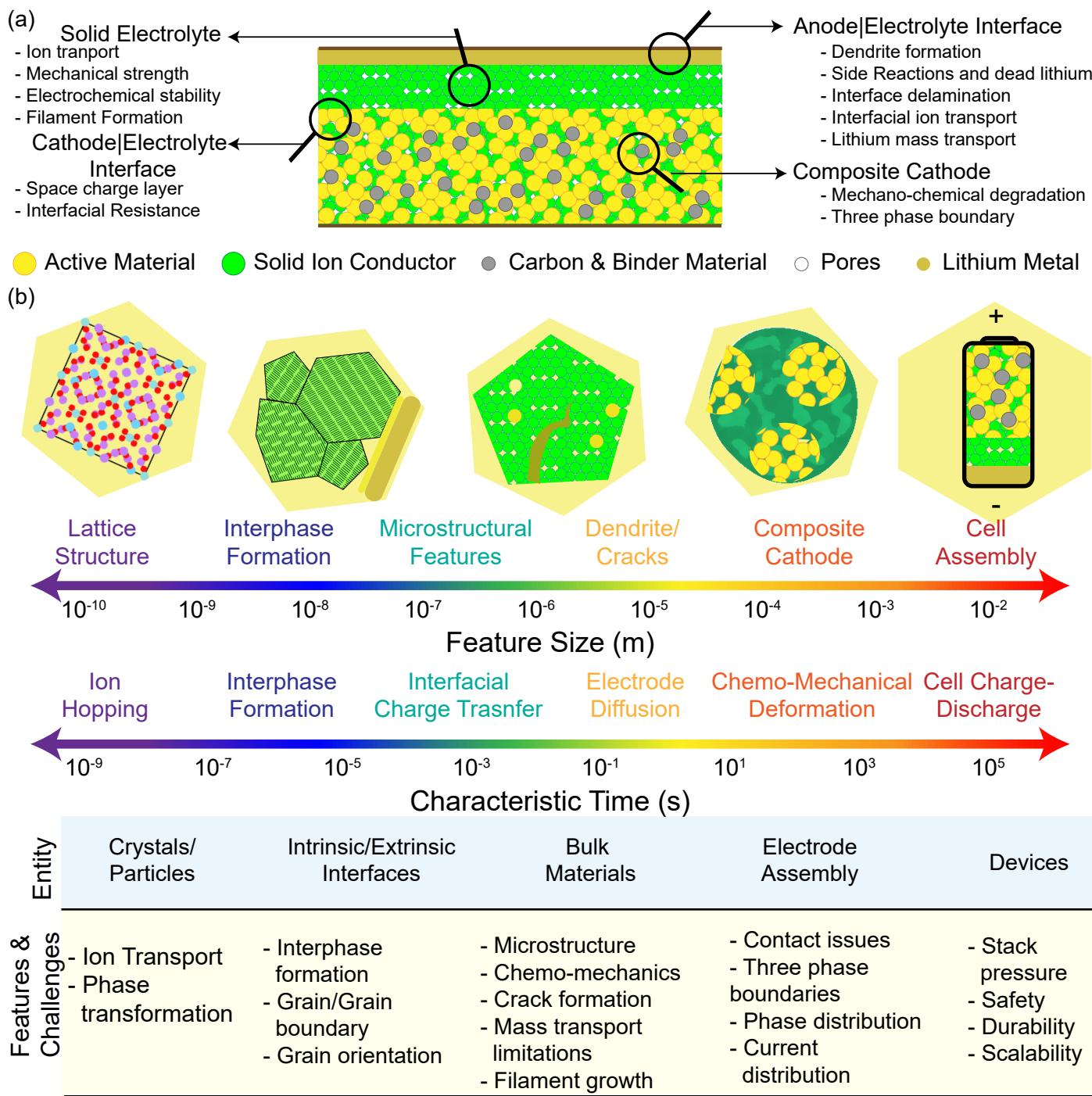
**Fig. 2** Summary of Challenges in Solid State Batteries. (a) Schematic diagram highlighting challenges at various components in a solid-state battery cell. (b) Temporal and spatial distribution of features and processes occurring in solid-state batteries. Physical entity in solid-state battery and corresponding features and challenges are also highlighted.
