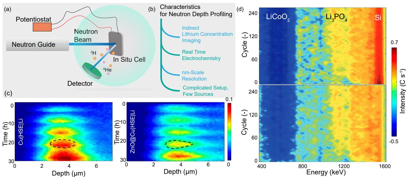
**Fig. 13** Summary of Neutron Depth Profiling Studies of Solid-State Batteries. (a) Schematic diagram showing the working principle of neutron depth profiling. (b) Characteristics of NDP studies. (c) Li plating in Cu|HSE|Li with and without a ZnO interlayer. Adapted with permission from<sup>163</sup>. Copyright 2020 American Chemical Society. (d) Lithiation and delithiation of LCO and Si electrodes. Adapted from<sup>164</sup> with permission from Wiley.
