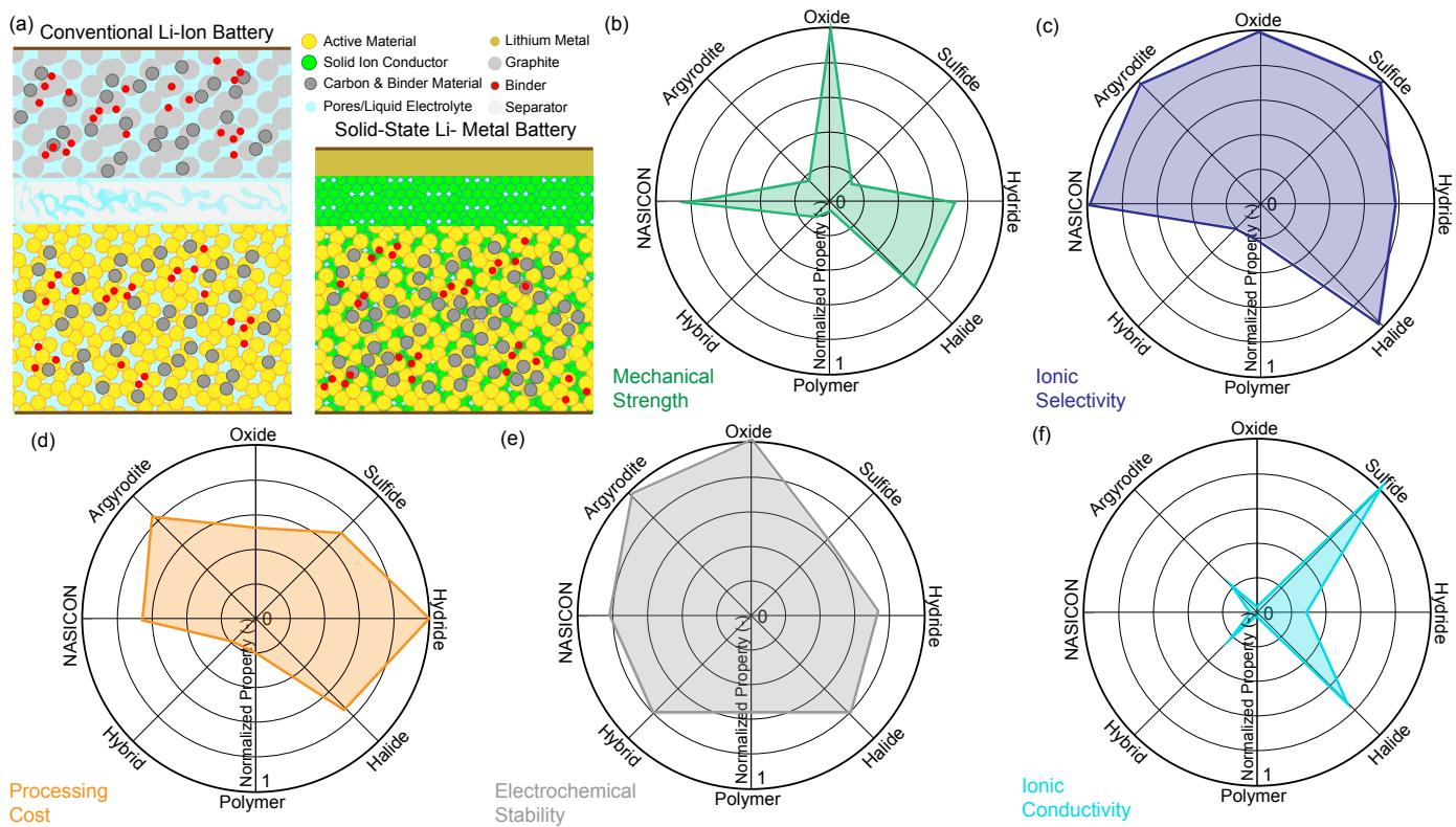
**Fig. 1** Solid-State Battery Technology Overview. (a) Schematic diagram showing differences in cell architecture between conventional Li-ion battery and solid-state Li metal battery. (b-f) Radar plot highlighting differences in material properties for a range of solid electrolyte materials. All physical quantities are normalized to one to enable comparison.
