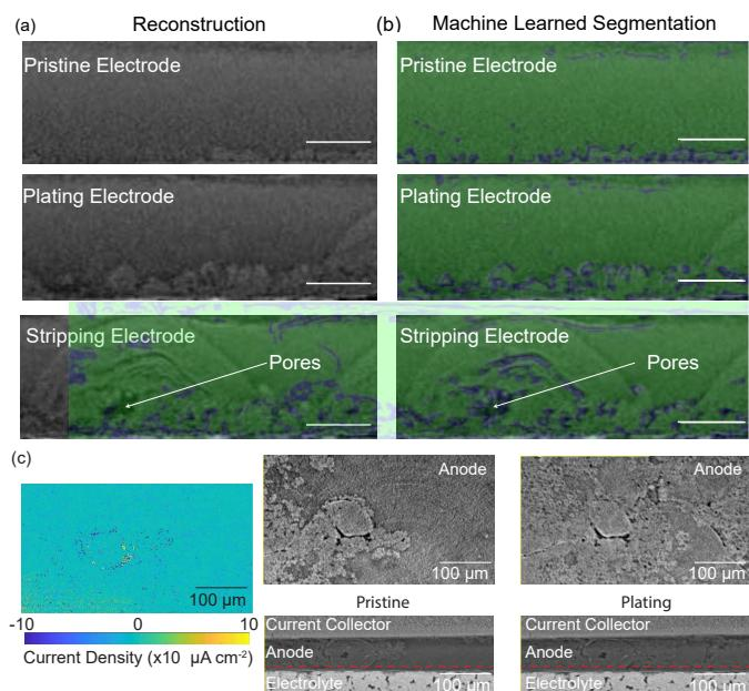
**Fig. 11** Li imaging by *in situ* XRT. (a) Raw XRT reconstructions for Li at different stages of cycling. Cross-section image shows evidence of hot-spot and pore formation in the Li electrode. (b) Convolution neural network enabled segmentation of Li and pore phases from the XRT images. (c) Local spatial current density maps highlighting hot spots in the Li metal and corresponding morphology. Adapted with permission from<sup>84</sup>. Copyright 2020 American Chemical Society.
