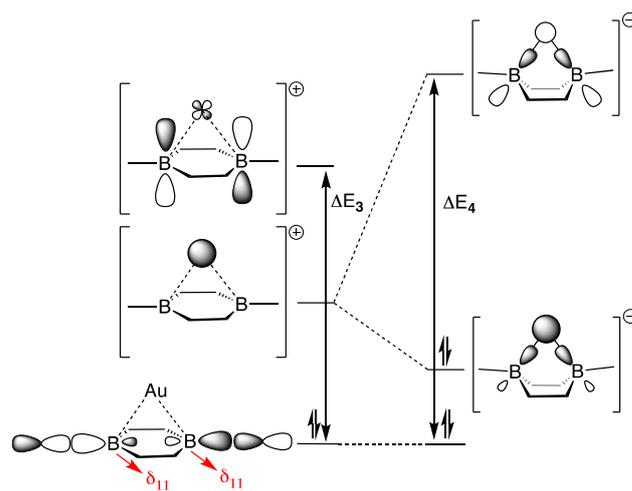
**Figure 7.** Qualitative molecular orbital diagram showing how  $\Delta E$  ( $\sigma^{p+SO}$ ) changes by adding two electrons to **3** (right diagram) to form **4** (left diagram).
