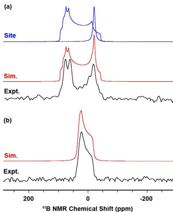
**Figure 4.** Static  $^{11}\text{B}\{^1\text{H}\}$  NMR spectrum of **3** (a) and **4** (b) acquired at 14.1 T. Experimental spectra are shown in black and simulated spectra are shown in red. The two simulated boron sites in **3** are shown in blue above the red simulated spectrum.**Table 3.**  $^{11}\text{B}\{^1\text{H}\}$  NMR data extracted from solid-state NMR measurements of **1–4**.<sup>a</sup>
