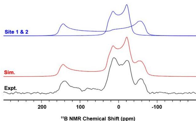
**Figure 2.** Static  $^{11}B\{^1H\}$  NMR spectrum of  $B_2P_2$  acquired at 9.4 T. Experimental spectra are shown in black and simulated spectra are shown in red. The two simulated boron sites in  $B_2P_2$  are shown in blue above the red simulated spectrum.
