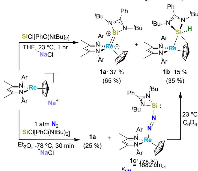
**Scheme 1.** Syntheses of complexes **1a-c**. Product ratios shown in parentheses are determined by <sup>1</sup>H NMR and isolated yields are shown without parentheses. Dinitrogen-bridged silylene **1c** decomposes to bridging silane **1b** in benzene-*d*<sub>6</sub> solution at ambient temperature over several days (no yield determined for this conversion).
