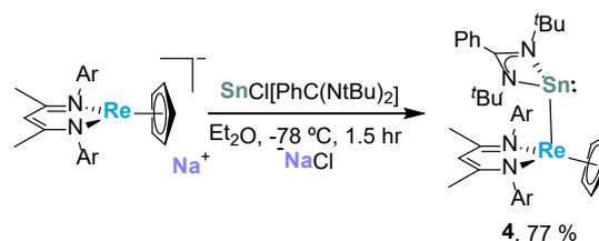
**Scheme 3.** Synthesis of  $\sigma$ -metallostannylene **4**. Gradual decomposition of **4** is observed in toluene- $d_6$  solution above ca.  $0^\circ\text{C}$  to form  $\text{Re}(\eta^5\text{-Cp})(\text{BDI})$ <sup>35</sup> and an unknown amidinate product.
