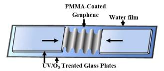
**Figure 1.** Schematic of folding process for PMMA-coated graphene in an accordion-like pattern. Glass plates were treated with  $UV/O_3$  prior to use. Wrinkles formed in the graphene sheet during compression along the width of the graphene sheet and remained folded as the sheet was compressed further.
