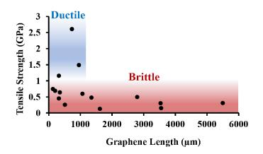
Figure 6. Breaking strength of parent and fragment fibers. Three fiber fragments exhibited ductile behavior and exhibited the largest measured breaking strengths. Brittle fracturing behavior was observed for most fibers.
