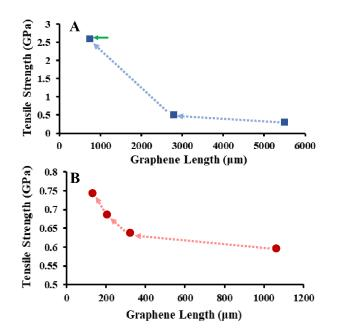
Figure 5. Breaking strength of graphene fibers as a function of fiber length. Dotted arrows indicate order of sequential uniaxial tensile tests on the same fibers with  $A_{graphene} = 3.2 \mu m^2$  (A) and  $A_{graphene} = 5.2 \mu m^2$ . (B). Green arrow indicates a measurement where ductile fracture behavior was observed during tensile testing.
