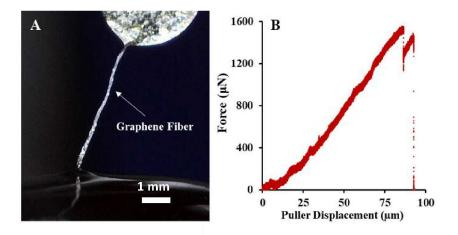
**Figure 3. Macroscale graphene fiber tested in uniaxial tension**. **A**, optical image of graphene fiber ( $A_{graphene}$ = 3.18 µm<sup>2</sup>,  $L_{fiber}$  = 2952 µm). **B**, Force-displacement plot of uniaxial tensile test (puller displacement rate  $r_p$ =0.50 µm/s). This fiber exhibited brittle fracture, with a tensile strength of 0.475 GPa.
