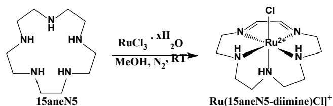
Scheme 2. Synthetic procedure for the synthesis of [\text{Ru}(\text{15aneN5-diimine})\text{Cl}]^+
