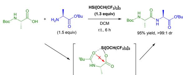
Scheme 20 HSi[OCH(CF<sub>3</sub>)<sub>2</sub>]<sub>3</sub>-mediated peptide bond-forming reaction.
