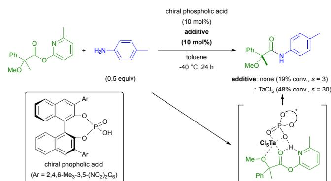
Scheme 19 Effect of tantalum catalysts in the chiral phosphoric-acid-catalysed kinetic resolution.
