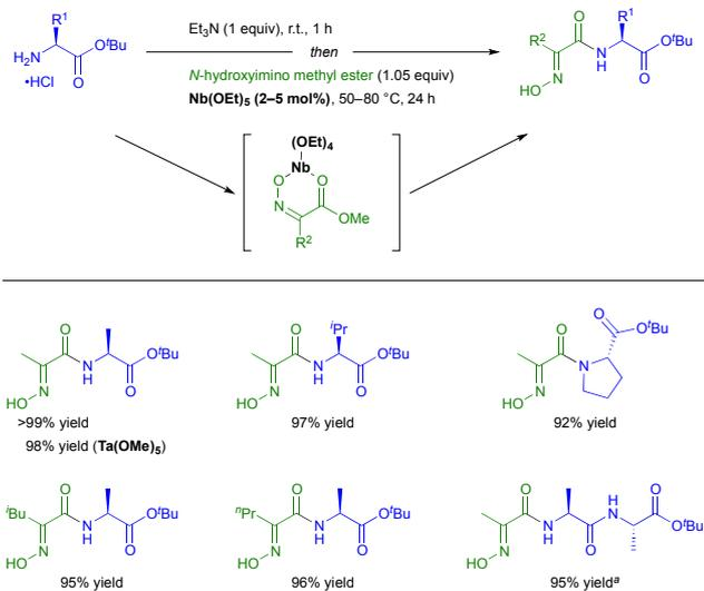
Scheme 12 Solvent-free hydroxy-group-directed amidation reaction using niobium catalyst. <sup>a</sup>Neutralisation using Et<sub>3</sub>N was omitted because H-L-Ala-L-Ala-O<sup>t</sup>Bu was employed.
