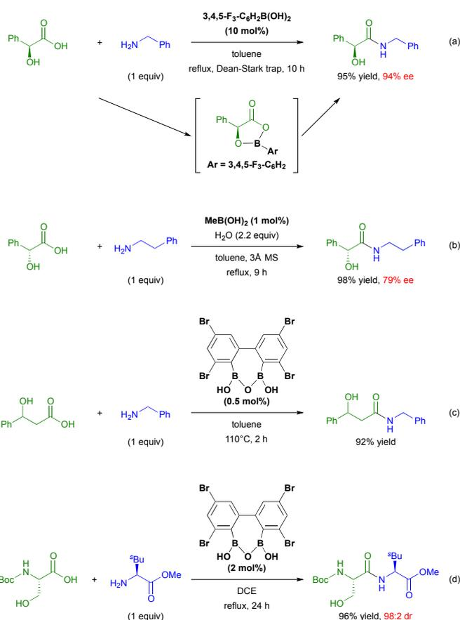
Scheme 9 Hydroxy-group-directed dehydrative amidation reaction using boronic acid catalysts.
