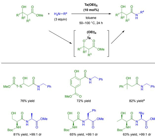
Scheme 15 Hydroxy-group-directed peptide bond-forming reaction using tantalum catalyst. <sup>a</sup>In the presence of methyl butyrate (1 equiv).
