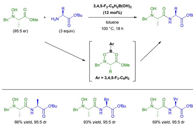
Scheme 10 Hydroxy-group-directed peptide bond-forming reaction using boronic acid catalyst.
