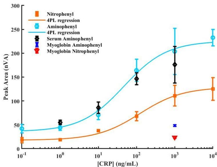
**Fig. 4.** CRP ELISA assay p-AP peak area data for reduced nitrophenyl (Nitrophenyl) modified electrodes and reduced aminophenyl (Aminophenyl) modified electrodes for various concentration of CRP in PBS buffer pH=7.4 (0.1-10<sup>4</sup> ng/mL; n=4 for all but PPD 10<sup>3</sup> ng/mL [n=3]), CRP spiked 100x diluted serum (1-10<sup>3</sup> ng/mL; n=3), and 10<sup>3</sup> ng/mL myoglobin (n=3).
