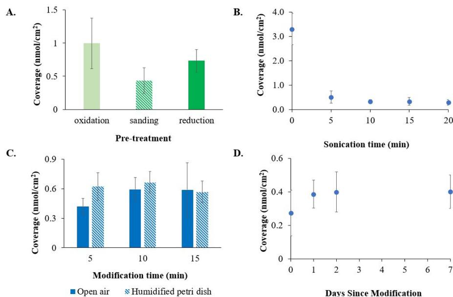
**Fig. 1.** P-nitroaniline modification optimization and stability testing. A) Pretreatment optimization (n=4), B) sonication time in IPA following modification (n=4), C) modification time and conditions: open air (5 and 10 min n=5; 15 min n=7) and humidified petri dish (5 min n=9; 10 and 15 min n=5), and D) Coverage stability.
