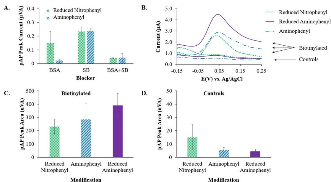
**Fig. 3.** Streptavidin-ALP assay data for reduced nitrophenyl, direct aminophenyl, and reduced aminophenyl modified electrodes from ALP generated p-AP SWV. A) Quantitative blocking optimization peak current data (BSA  $n=6$ ; SB and BSA+SB  $n=3$ ), B) averaged voltammograms for biotinylated TPEs and unbiotinylated controls (biotinylated  $n=6$ ; controls  $n=3$ ), C) quantitative peak area data for biotinylated electrodes, and D) quantitative peak area data for unbiotinylated controls.
