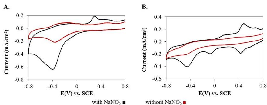
**Fig. 2.** Averaged cyclic voltammetry of modified 1 mm diameter TPEs in  $N_2$  degassed  $0.1 M H_2SO_4$ ,  $v=100$  mV/s, modified with and without  $NaNO_2$ . A) p-nitrophenyl diazonium salt modification (with  $NaNO_2$   $n=16$ ; without  $NaNO_2$   $n=6$ ), B) p-aminophenyl diazonium salt modification (with  $NaNO_2$   $n=6$ ; without  $NaNO_2$   $n=6$ ).
