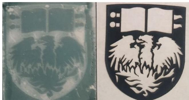
**Fig. 6** A pattern of **M1** (left) and the laser cut black mask (right).
