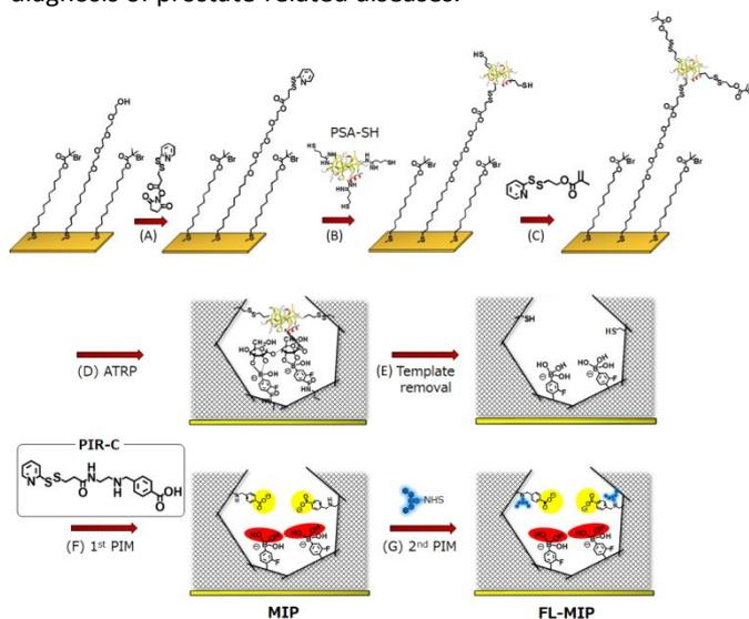
**Figure 2.** Synthesis procedure of molecularly-imprinted polymer (MIP) thin layer possessing orthogonal dual interaction sites and fluorescent reporting groups via molecular imprinting and sequential post-imprinting modifications (PIMs).
