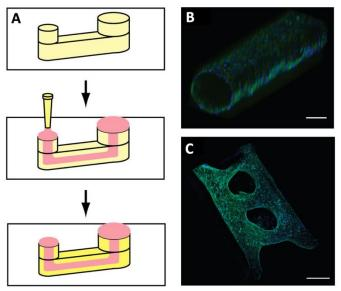
**Figure 6.** Viscous Finger Patterning. **A)** Passive pumping technique for the on-chip fabrication of lumen. Channels are first filled with an unpolymerized gel; less viscous cell media is then passively pumped through the gel and the gel is then polymerized. **B, C)** Confocal images of single (B) and multi-lumen (C) constructs with endothelial cells. Scale bars are 100 $\mu$ m (B) and 500 $\mu$ m (C). (A) – (C) reproduced with permission from ref 100: Copyright (2013) Elsevier.
