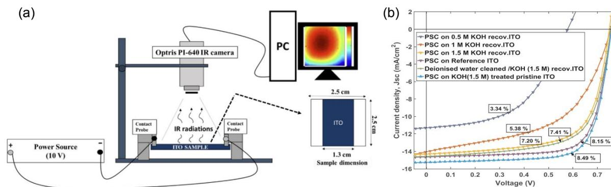
**Fig. 4.** Schematic the set-up of synchronized thermography for sample surface electrical uniformity by corresponding IR distribution (a).  $J$   $V$  curves (reverse scan) of PSCs before and after recycling the ITO/glass substrate of the best working devices (b). Copyright 2019, Elsevier Inc.
