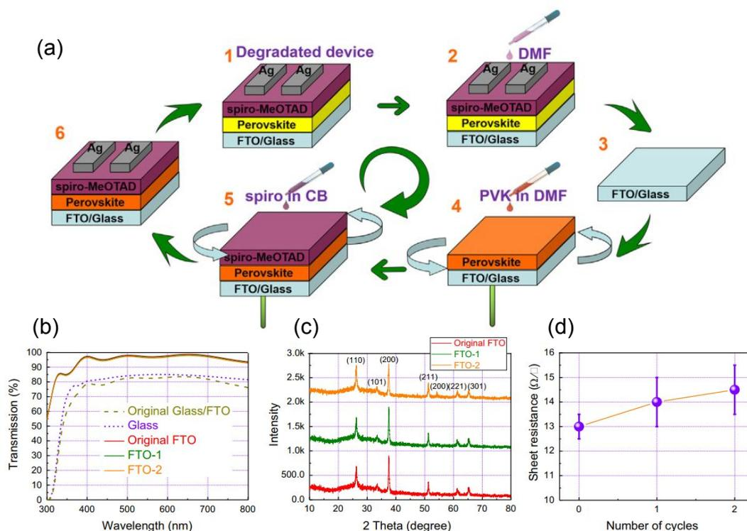
**Fig. 2.** (a) Schematic demonstration of process to fabricate PSCs with ETL-free via recycling the FTO/glass substrates. (b) Optical transmission spectra, (c) X-ray diffraction (XRD) patterns and (d) Sheet resistance of fresh, one-time (FTO-1) and two-times (FTO-2) recycled FTO/glass substrates. Copyright 2016, Elsevier Inc.
