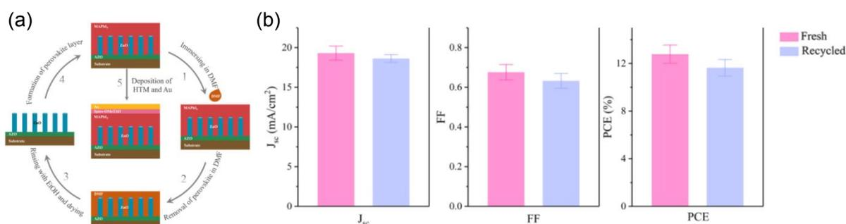
**Fig. 7.** Schematic of recycling process of ZnO/AZO substrates (a),  $V_{OC}$ ,  $J_{SC}$ , FF and PCE of six PSCs devices before and after recycling. Copyright 2018, Wiley-VCH.
