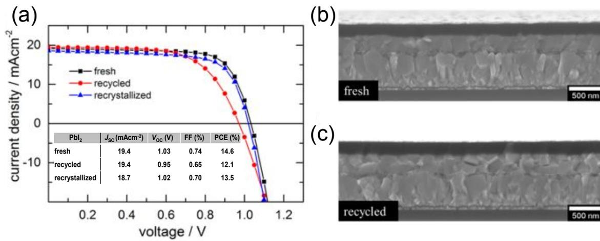
**Fig. 9.** (a)  $J$  -  $V$  curves of PSCs fabricated from fresh, recycled and recrystallized  $\text{PbI}_2$  after recycling. (b) and (c) SEM cross-sectional images of PSCs on fresh and recycled  $\text{PbI}_2$ . Copyright 2016, American Chemical Society.
