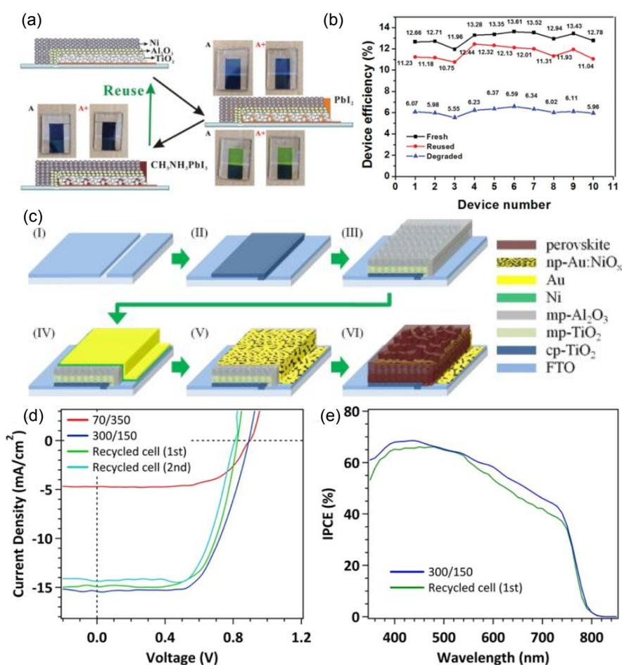
**Fig. 12.** Schematic of recycling process of m-NiO electrode PSCs (a), PCE distribution of PSCs with 10 devices under various condition: fresh, reused and degraded (b). Copyright 2015, The Royal Society of Chemistry. Illustration of the monolithic structure PSCs fabrication process. (I) Etching FTO substrate; (II) compact TiO<sub>2</sub> (cp-TiO<sub>2</sub>) spray loading; (III) mp-TiO<sub>2</sub> spin coating; (IV) thermal deposition of Ni/Au
