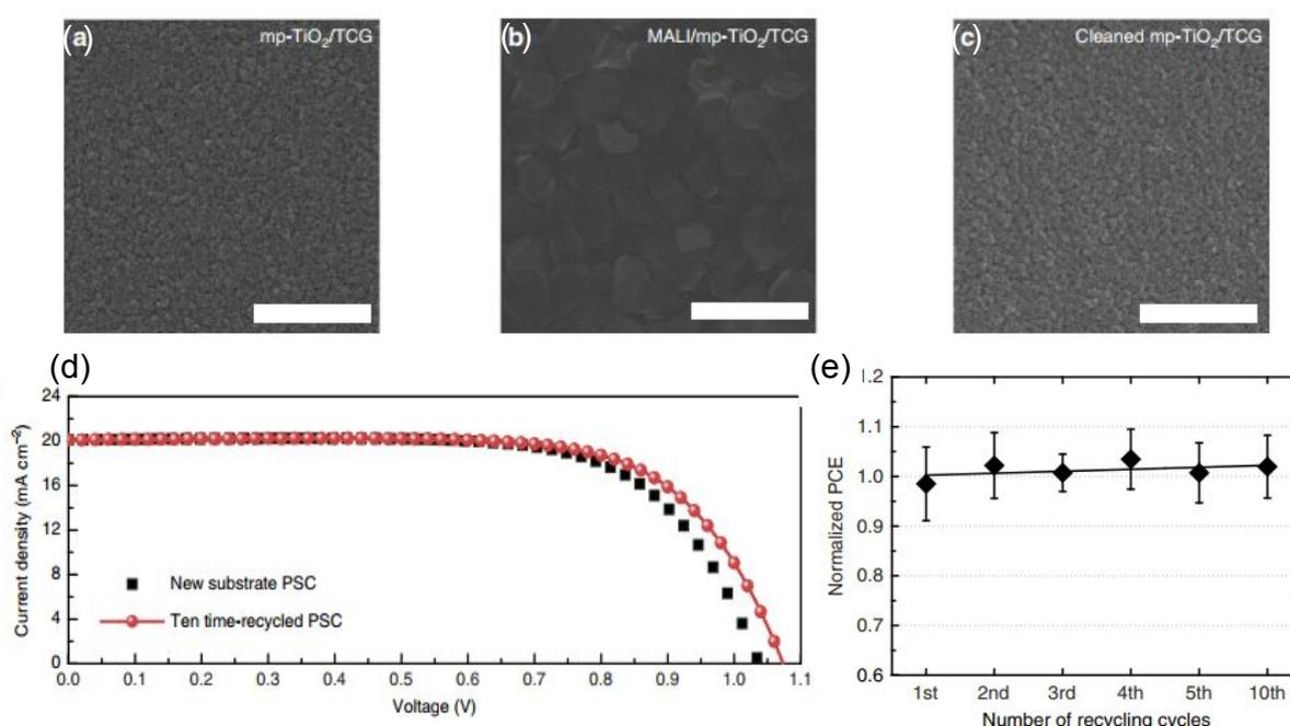
**Fig. 5.** SEM images of fresh mp- $\text{TiO}_2$  film on FTO/glass (a),  $\text{MAPbI}_3$ -perovskite on the top of  $\text{TiO}_2$  (b), and recycled  $\text{TiO}_2$  film after using DMF as dissolving solvent (c). The scale bar is 1  $\mu\text{m}$ . TCG:
