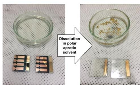
**Fig. 10.** Optical images of PSCs before and after selectively dissolution. The yellow color metal is Au electrode. Copyright 2016, Springer Nature.
