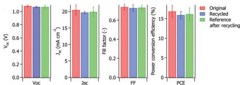
**Fig. 6.** Photovoltaic parameters summarization of PSCs on fresh, first- and second-times recycled mp-TiO<sub>2</sub>/FTO/glass substrates. Copyright 2016, The Royal Society of Chemistry.
