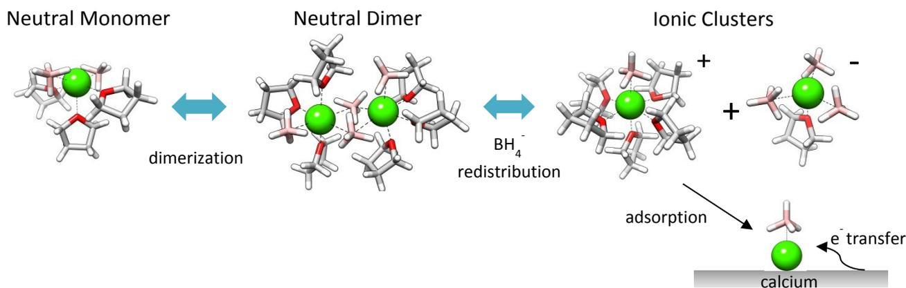
**Scheme 1.** Reaction pathway for ionic cluster formation in the THF<sub>n</sub>Ca(BH<sub>4</sub>)<sub>2</sub> electrolyte system yielding CaBH<sub>4</sub><sup>+</sup> as the species responsible for Ca electrodeposition.
