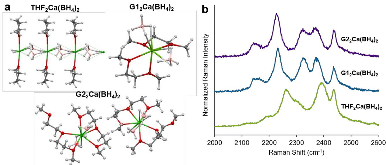
**Figure 4.** a) Solvate crystal structures determined through single crystal XRD. The G2 solvate structure comes from data generated in Ref. 59 while the THF and G1 structures were determined in this work. b) Raman  $\nu(\text{B-H})$  spectra for the indicated solvate crystals.
