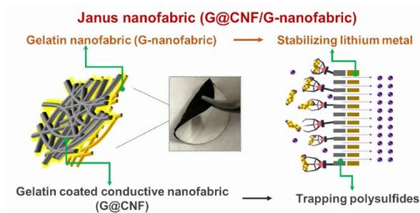
A protein-based, low-resistance Janus nanofabric is designed and fabricated for simultaneously trapping polysulfides and stabilizing lithium metal.
