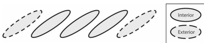
Fig. 3 Classifying particle chains: particles in the chain are labelled as either interior or exterior particles, depending on location.
