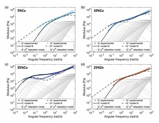
Fig. 6 Comparison between experimental data and fitting results by applying the enhanced sticky Rouse model: (a) 5%Cu, (b) 10%Cu, (c) 25%Cu, and (d) 25%Zn. The thin grey lines show the relaxation modes in Eq. 9 that add up to form the overall simulation response.
