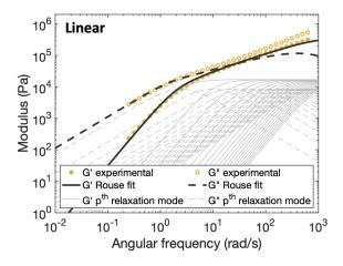
Fig. 4 Comparison between experimental data and fitting results of the Rouse model for the linear polymer. The thin grey lines show the relaxation modes in Eq. 4 (solid lines for G' and dashed lines for G'') that add up to form the overall simulation response.
