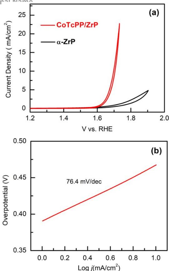
**Figure 5.** (a) Cyclic voltammograms of CoTcPP/ZrP and  $\alpha$ -ZrP on a rotating disk electrode in 0.1 M KOH aqueous solutions. Scan rate: 10 mV/s. Both CoTcPP/ZrP and  $\alpha$ -ZrP were modified with carbon black to enhance conductivity; (b) Tafel plot of CoTcPP/ZrP.
