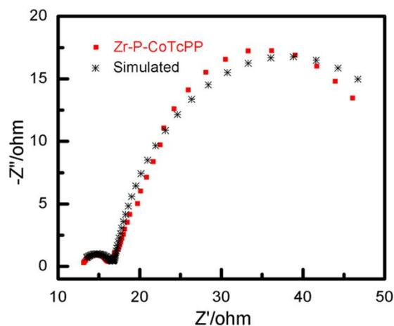
**Figure 8.** Electrochemical impedance spectroscopy and simulation fit spectra of the oxygen evolution reaction on the
