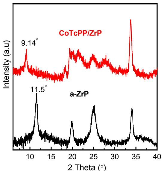
**Figure 3.** X-ray powder diffraction patterns of  $\alpha$ -ZrP and CoTcPP/ZrP.
