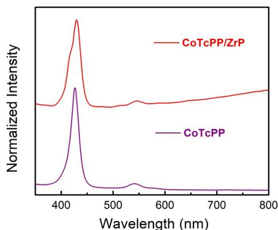
**Figure 2.** Overlaid UV-Vis spectra of CoTcPP in ethanol solution and CoTcPP/ZrP in ethanol suspension. The absorption spectrum of CoTcPP/ZrP was baseline corrected.
