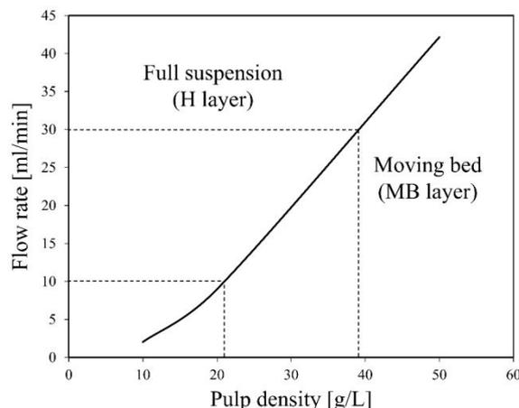
Fig. 2 Flow pattern map of LiCoO<sub>2</sub> slurry.
