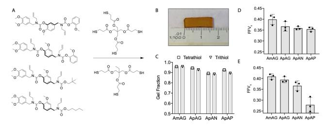
Figure 4. (A) Macromer cross-linking via a photo-initiated thiol-ene reaction with a tetrathiol and trithiol. (B) Image of crosslinked film (C) Gel fraction for each of the crosslinked networks after 60 minutes of irradiation. Fractional free volume of static holes (FFV<sub>h</sub>) of macromers crosslinked with the (D) tetrathiol, and (E) trithiol cross-linker.
