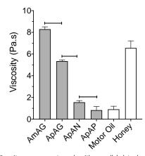
Figure 3. Viscosity measurements made with a parallel plate rheometer at a temperature of 45 °C and a constant shear rate of 0.1  $s^1$ . \*\*\*, p-value < 0.0001, \*, p-value < 0.05
