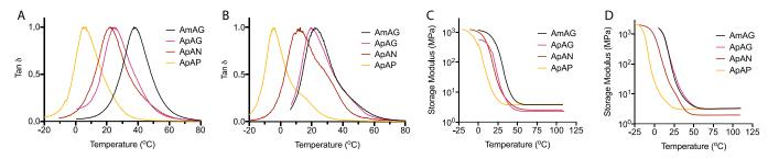
Figure 6. Thermal and mechanical properties of sequence defined networks (60 min. UV-cure). (A–D) Dynamic mechanical analysis of cross-linked networks. The tan δ curves of networks cross-linked with (A) tetrathiol and (B) trithiol. Plots of storage modulus (log scale) as a function of temperature for (C) tetrathiol cross-linked networks and (D) trithiol cross-linked networks.
