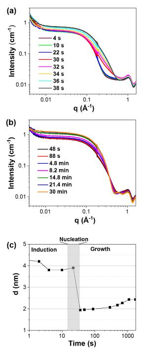
**Figure 5.** *In situ* SAXS patterns recorded during the synthesis of Au nanoparticles in OY/hexane solution with [OY] = 50 mM: (a) between 4 and 40 s and (b) between 48 s and 30 min; (c) Particle mean diameter as a function of time, calculated from the radius of gyration of the Au(III)-Au(I) pre-nucleation clusters during the induction stage and from that of Au(0) NPs during the growth stage. The grey shaded area corresponding the nucleation stage was deduced from the XAS results.
