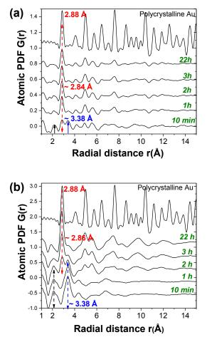
**Figure 8.** *In situ* atomic PDFs as a function of time: (a) [OY] = 100 mM; (b) [OY] = 400 mM. The blue arrow highlights the Au-Au pair distances present at the beginning of the reaction as a PDF peak centered at 3.38 Å; the black arrow highlights the bonds between Au and light atoms, N or Cl, appearing as a broad PDF peak centered at about 2.15 Å; the red dotted arrow highlights the Au-Au pair distances in metal NPs appearing as a well-defined PDF peak centered at 2.84 Å and 2.86 Å.
