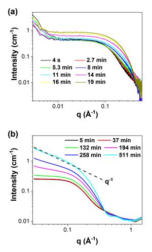
**Figure 7.** *In situ* SAXS patterns recorded during the synthesis of Au nanoparticles in OY/hexane solution: (a) [OY] = 100 mM, during the first 20 minutes and (b) [OY] = 400 mM.
