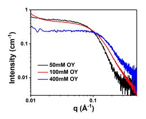
**Figure 3.** SAXS pattern of the initial precursors obtained by dissolving  $HAuCl_4$  in solution of OY in hexane at the OY concentrations of 50 mM (black line), 100 mM (red line) and 400 mM (blue line).
