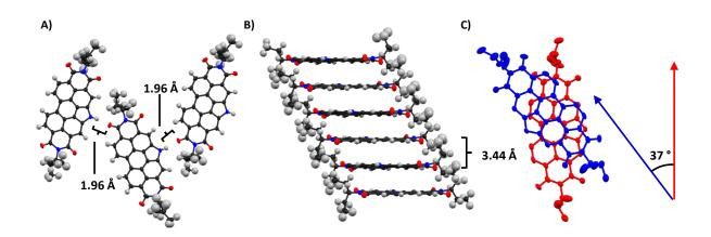
**Figure 8.** Structural of PDIN-H highlighting: A) hydrogen bonding between the NH and C=O functional groups, B)  $\pi$ - $\pi$  stacking motif, and C) the offset and dihedral angle
