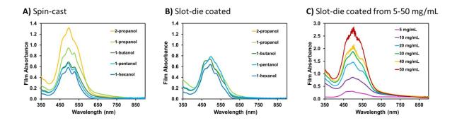
**Figure 5.** Optical absorption spectra of A) PDIN-H films spin-coated from different alcohols at 10 mg/mL, B) PDIN-H films slot-die coated from different alcohols at 10 mg/mL, and C) PDIN-H films slot-die coated from 1-propranol at varying concentrations onto PET. In all cases 1 molar equivalent NaOH was added to each pre-deposition solution.
