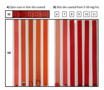
**Figure 4.** A) Top – images of spin-coated (SC) 1.5 cm x 1.5 cm films. Bottom – images of slot-die coated (SD) 13 mm x 20 cm films., (1) 2-propanol, (2) 1-propanol, (3) 1-butanol, (4) 1-pentanol, (5) 1-hexanol. Films prepared from 10 mg/mL solutions of PDIN-H in
