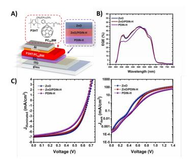
**Figure 9.** A) OPV device architecture. B) EQE spectra. C) Current density-voltage characteristics under 1-sun illumination (left) and in the dark (right). PDIN-H layer processed from PDIN-H solutions in 1-propanol with 1 molar equivalent of NaOH added.
