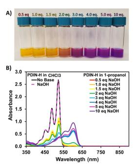
**Figure 2.** A) Image showing the color changes of PDIN-H in 1-propanol solution with varying equivalents of NaOH added. B) UV-vis spectra of PDIN-H solutions in CHCl<sub>3</sub> with 1 mol equivalent NaOH, and in 1-propanol with 0-10 mol equivalents of NaOH.
