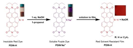
**Figure 1.** Chemical structure of PDIN-H. Treatment of a 10 mg/mL slurry of PDIN-H in 1-propranol with 1 molar equivalent of NaOH produces a purple ionic solution. Spin-coating this solution onto a PET substrate yields a red colored organic film owing to the spontaneous protonation of the PDIN anion. This processes mimics that of classic acid dyeing of textiles.
