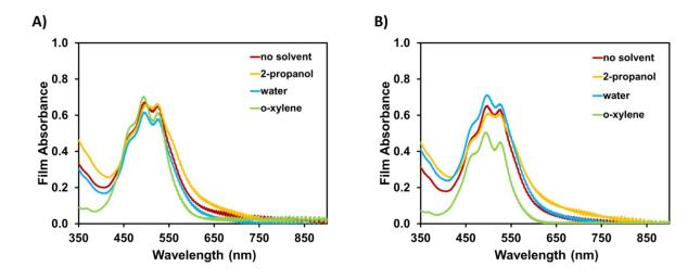
**Figure 7.** Optical absorption spectra of PDIN-H films as-cast with no solvent coated on top and with A) 2-propanol, water, or o-xylene slot-die coated on top and left to dry or B) dipped in 2-propanol, water, or o-xylene for 10 s then removed and left to dry.
