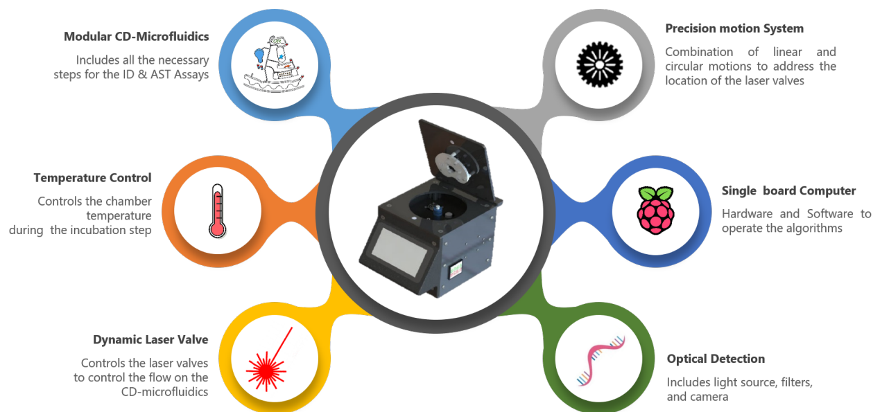
Fig. 1 The SpinBox design and components.
