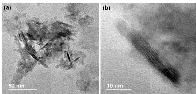
**Figure 1.** Transmission electron micrographs of pristine LiCoO<sub>2</sub> nanoparticles.
