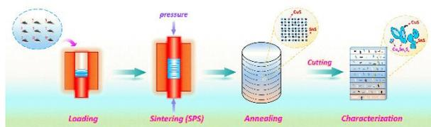
A modified HTP synthesis method and an automated histogram analysis technique are developed to screen the new stable ternary CTS compound  $\text{Cu}_7\text{Sn}_3\text{S}_{10}$ .
