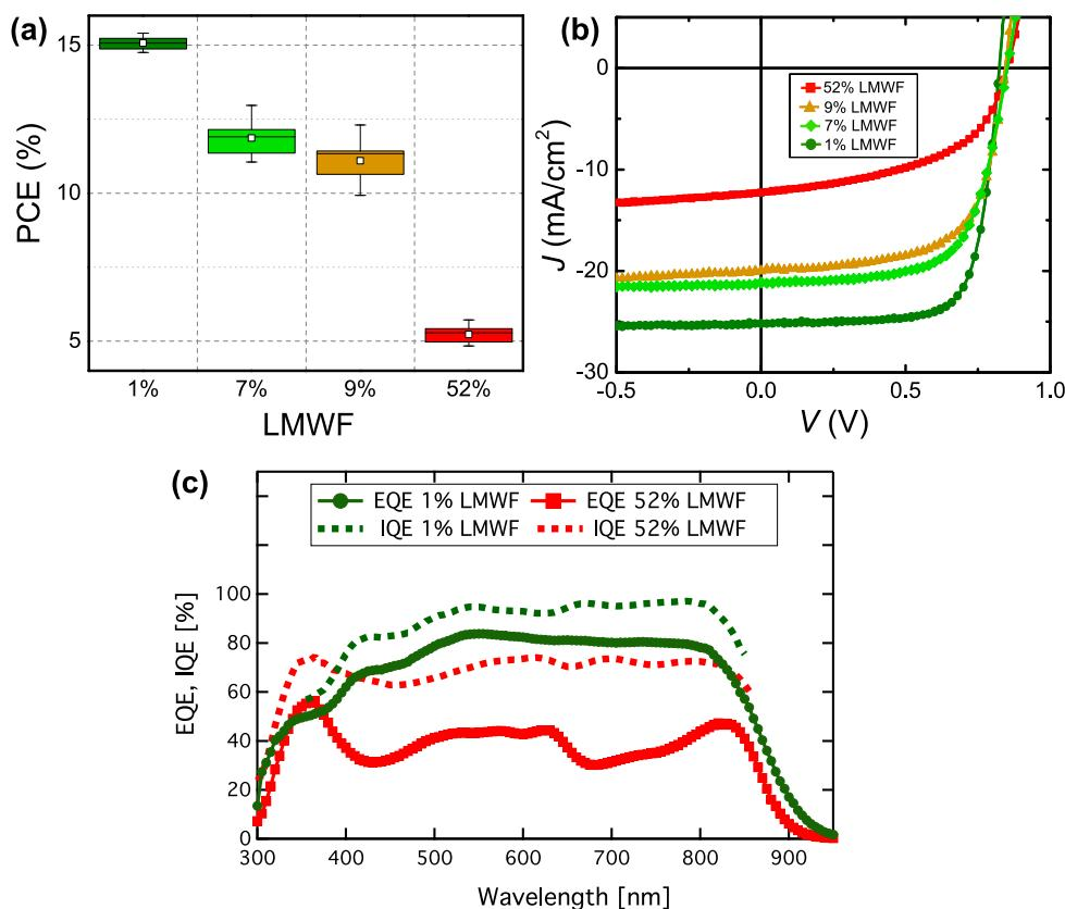
**Fig. 2** (a) Box plots showing PCE averages for the 1%, 7%, 9%, and 52% LMWF PM6:Y6 blends. (b)  $J$ - $V$  curves of the 1%, 7%, 9%, and 52% LMWF PM6:Y6 blends and (c) EQE and
