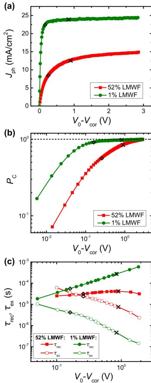
**Fig. 6** (a) Photocurrent  $J_{\text{ph}}$  and (b) collection probability  $P_C$  of the 1% and 52% LMWF PM6:Y6 batches. (c) Average extraction time  $\tau_{\text{ex}}$  and charge carrier lifetime  $\tau_{\text{rec}}$  of the two batches.
