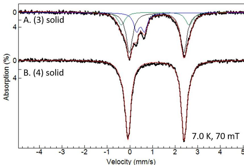
**Figure 4.** MB spectra of complexes **3** and **4** measured at 7.0 K and 70 mT. The samples were prepared by suspension of powders in degassed mineral oil. The hatch marks are the experimental data, and the colored lines are spectral fits generated with the parameters in Table 2. For clarity, in spectrum A an unknown species with  $\delta = 0.75$  and  $\Delta E_Q = 1.0$  mm/s accounting for 5% absorption was subtracted from the raw data.
