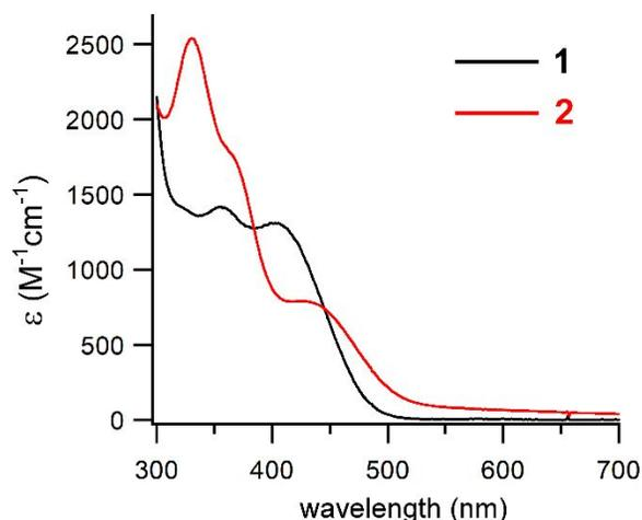
**Figure 6.** UV-vis absorption spectra of **1** and **2** in  $\text{CH}_2\text{Cl}_2$  at room temperature.
