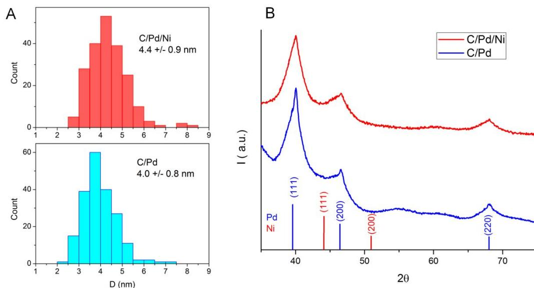
Figure 2: (A) Particle size distribution (PSD) and (B) Powder X-ray diffraction (PXRD) patterns of the catalysts (Pd and Ni reflections marked by solid lines).
