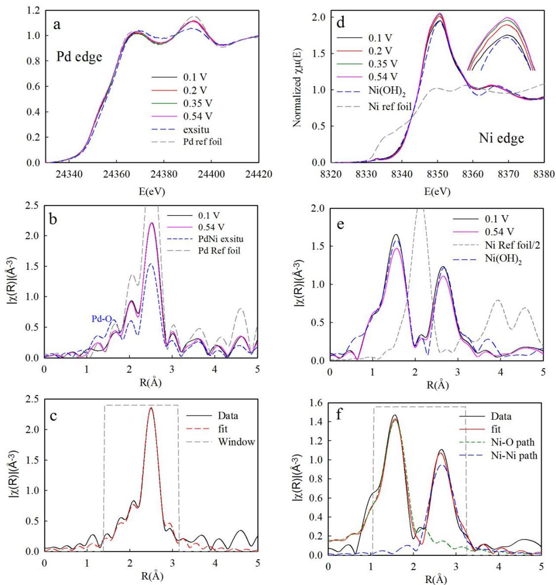
Figure 5. The *ex situ* and *in situ* XANES spectra at the Pd (a) and Ni (d) edges; the *in situ* FT-EXAFS spectra at the Pd (b) and Ni (e) edges; and the EXAFS fitting of the Pd (c) and Ni (f) edges of Pd/ $\gamma$ -NiOOH.
