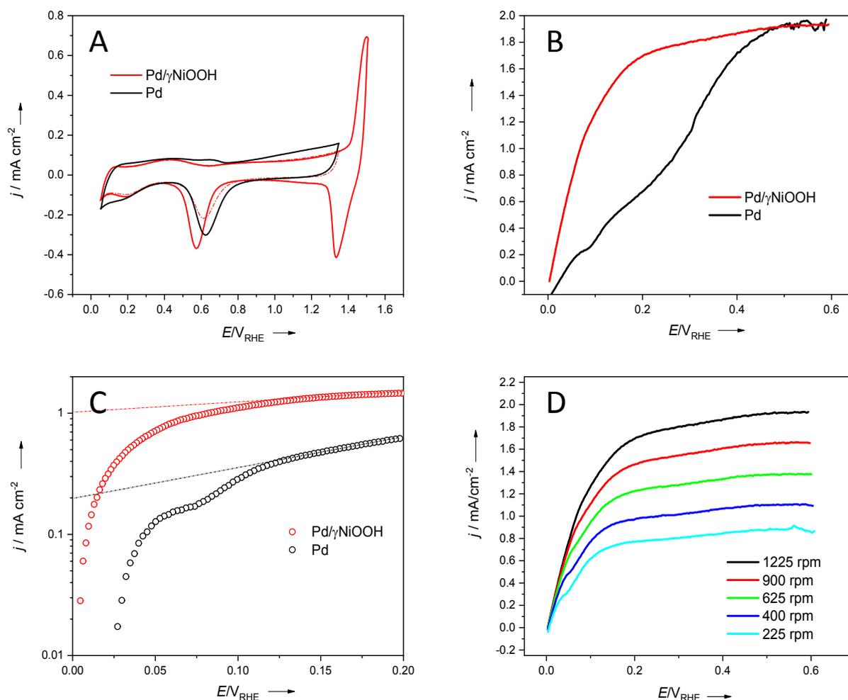
Figure 3: (A) Cyclic voltammograms recorded at 298 K in an Ar-saturated 0.1 M KOH solution; (B) Ohmic loss corrected cathodic polarization at 298 K in an  $H_2$ -saturated 0.1 M KOH solution at 1225 rpm; (C) corresponding Tafel plot and (D) Pd/γ-NiOOH at different rotation speeds.
