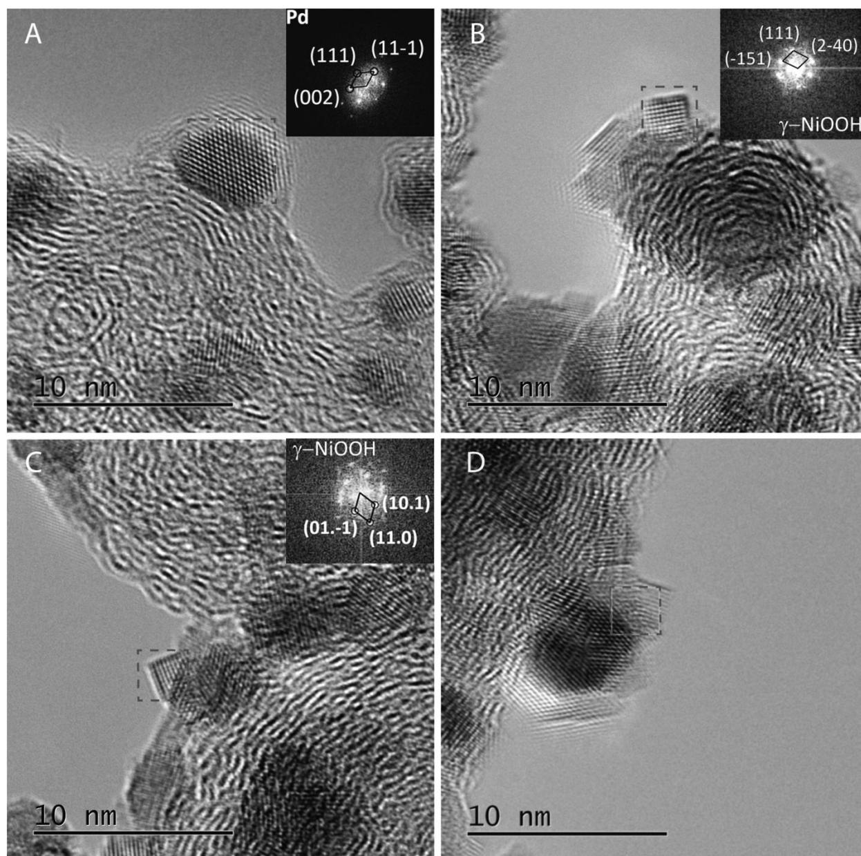
Figure 1: High-Resolution Transmission electron microscopy (HR-TEM) of the Pd and Pd/ $\gamma$ -NiOOH samples: (A) Pristine Pd samples with Fast-Fourier Transform (FFT) (inset); (B-D) HRTEM images of Pd/ $\gamma$ -NiOOH with corresponding FFT (insets).
