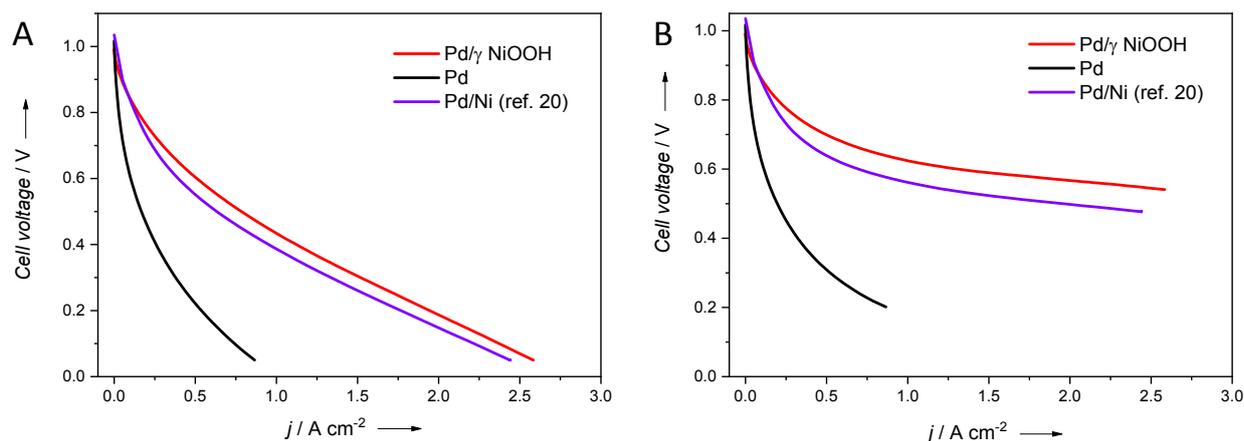
Figure 4: (A) Raw and (B) IR-corrected polarization curves of MEAs with different anode catalysts, Pd/ $\gamma$ -NiOOH (red), Pd (black) and Pd/Ni composite from ref. 20 (purple).
