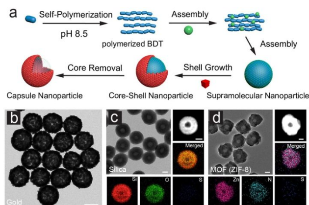
Fig. 17 (a) Synthetic strategy for particle engineering using pBdT-TA supramolecular networks. The polyphenol-stabilized particles subsequently allow for the growth of diverse shell materials on the particles. TEM images of (b) Au (c) silica, and (d) MOF hollow structures after removal of the pBdT-TA core. Insets in image c and d: HAADF-STEM images of representative silica and MOF hollow particles and their corresponding EDX mapping results. Reproduced with permission. Copyright 2020, Nature Publishing Group.
