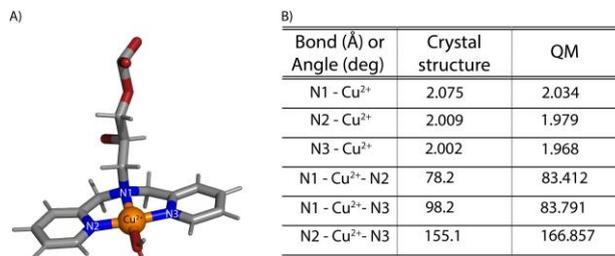
**Figure 3:** A) DFT optimized structure of Cu<sup>2+</sup>-DPA B) Comparison of bond angles and bond lengths with crystal structure<sup>80</sup> of Cu<sup>2+</sup>-DPA show reasonable agreement with the DFT-optimized structure.
