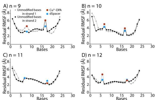
**Figure 9:** The root mean square fluctuations (RMSF) of all the bases in the Cu<sup>2+</sup>-DPA-DNA duplexes with A) n=9 B) n=10 C) n=11 and D) n=12. The grey and black denote the two strands in the DNA and the red and blue denote Cu<sup>2+</sup>-DPA and dSpacer, respectively. As can be seen, the RMSF is high for the terminal bases, as expected. The RMSF for Cu<sup>2+</sup>-DPA and the abasic dSpacer positions are generally high, indicating more flexibility than the natural bases.
