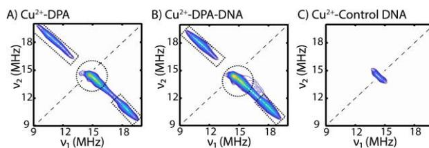
**Figure 4:** <sup>1</sup>H HYSCORE spectra of A) Cu<sup>2+</sup>-DPA B) Cu<sup>2+</sup>-DPA-DNA and C) Cu<sup>2+</sup>-control DNA, analysed to the same contour levels. In Cu<sup>2+</sup>-DPA and Cu<sup>2+</sup>-DPA-DNA, the proton signal results from equatorially coordinated water molecule (rectangle) and weakly coupled solvent (circle). In control DNA, the proton signal results from only weakly coupled solvent molecules.
