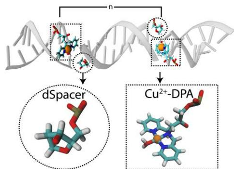
**Figure 1:** Cu<sup>2+</sup>-DPA-DNA duplex with the Cu<sup>2+</sup>-DPA motif (highlighted by a rectangle) and the dSpacer (highlighted by a circle). The base pair separation between the two Cu<sup>2+</sup>-DPA motifs is denoted by n.
