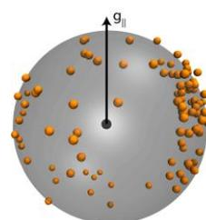
**Figure 16:** MD frames of  $\text{Cu}^{2+}$ -DPA-DNA duplex ( $n=11$ ) sampled every 10 ns for the first 1  $\mu\text{s}$ . The black sphere in the center is the reference  $\text{Cu}^{2+}$ . All frames are aligned to the  $g_{\parallel}$  axis of the reference  $\text{Cu}^{2+}$ . The second  $\text{Cu}^{2+}$  position is represented as orange spheres. The  $g_{\parallel}$  direction, marked in the figure, is calculated from ORCA<sup>105,106</sup>.
