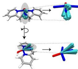
**Figure 14:** The distribution of  $g_{\parallel}$  directions (cyan) in the  $\text{Cu}^{2+}$ -DPA system, sampled every 10 ns of the 1  $\mu\text{s}$  MD run. The blue and red bonds show the  $\text{Cu}^{2+}$  coordination with nitrogen and oxygen, respectively. The cyan represents the  $g_{\parallel}$ . The  $g$ -tensor calculations were performed with ORCA<sup>105,106</sup>.
