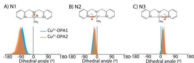
**Figure 13:** Dihedral angles measured between  $\text{Cu}^{2+}$  and its coordinating atoms for 2  $\mu\text{s}$  of MD run on  $\text{Cu}^{2+}$ -DPA-DNA duplex with  $n=11$ . The dihedral angle is denoted by the red arrow (top chart). Bottom chart shows the probability distribution of the dihedrals between the two  $\text{Cu}^{2+}$ -DPA sites,  $\text{Cu}^{2+}$ -DPA1 (blue) and  $\text{Cu}^{2+}$ -DPA2 (orange).
