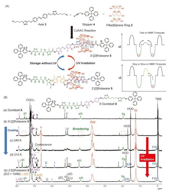
**Fig. 2** (A) Synthesis of pillar[6] arene-based [2] rotaxane **5** from pillar[6] arene ring **2**, stopper **4** and azobenzene axle **3**. (B)  $^{1}$ H NMR spectra (CDCl $_{3}$ ) of (a) dumbbell **6** at 298 K, (b-d) E-[2] rotaxane **5** at different temperatures and (e) Z-[2] rotaxane **5** (E/Z = 10/90) at 298 K.
