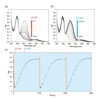
Fig. 4 Absorption spectra of [2] rotaxane 5 (25  $\mu$ M in CHCl<sub>3</sub> at 298 K) (a) during UV light irradiation, and (b) subsequent recovery in the dark. (c) Absorbance change at 357 nm accompanying the *E*-to-*Z* conversion of [2] rotaxane 5 (25  $\mu$ M in CHCl<sub>3</sub> at 298 K) by UV irradiation in a 120 s/2000 s light-dark cycle.
