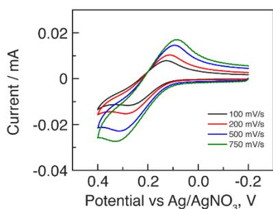
**Figure 4.** Scan rate dependence of the initial oxidation event in cyclic voltammograms of  $\text{Fe}_3(\text{TPM})_2$  under  $\text{N}_2$  (0.7 mM  $\text{Fe}_3(\text{TPM})_2$ , 0.1 M  $\text{NBu}_4\text{PF}_6$ ). Potential is referenced vs.  $\text{Ag}/\text{AgNO}_3$  ( $\text{Fc}^{\text{O}^+}/\text{Fc}^{\text{O}}$   $E_{1/2} = 0.257$  V vs.  $\text{Ag}/\text{AgNO}_3$ ).
