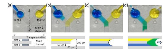
Figure 2 Sequential images and side-sectional schematics of the simultaneous inflow system at the moments of (a) pipetting the solutions, (b) arriving the junction, (c) making a combined meniscus, and (d) entering into the main channel.
