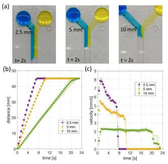
Figure 5 (a) Y-shape devices with three different inlet length channels. All images show 2 s after blue and yellow dyes begin to flow through the main channel. (b) Flow distance in the main channel and (c) velocity variations over time for three different inlet channel devices. All data were calculated every 0.5 s and indicate the average (symbol) with the standard deviation (error bar) for three repeated experiments.
