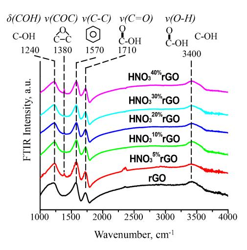
Figure 4. FTIR spectra of the initial and HNO<sub>3</sub>-treated rGO materials.
