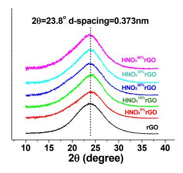
**Figure 6.** XRD patterns of the initial and  $HNO_3$ -treated rGO materials.
