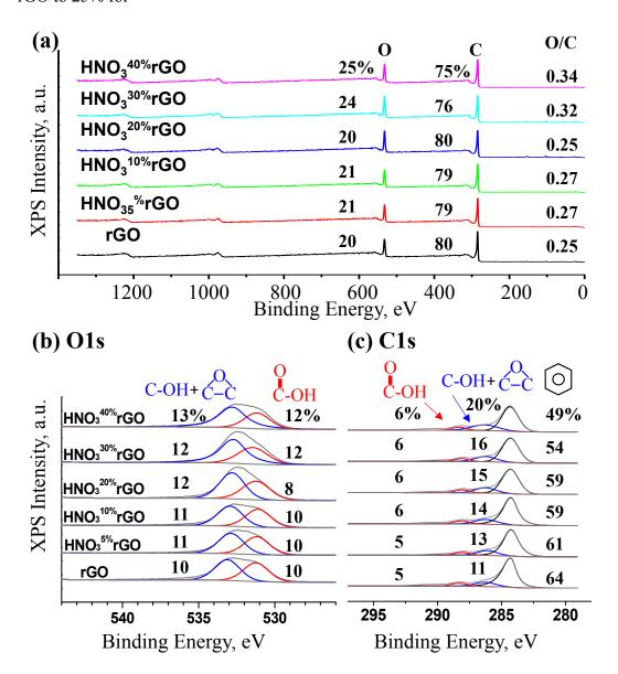
**Figure 5.** XPS spectra of the initial and HNO<sub>3</sub>-treated rGO materials.
