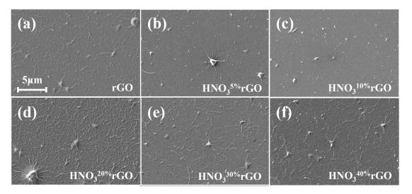
Figure 2. SEM images of (a) rGO and (b-f)  $HNO_3$ -treated rGO films on Si wafers.
