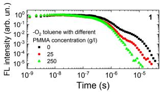
Fig. 5 Fluorescence decay transients of compound 1 at  ${}^{1}CT_{2}$  peak in oxygen-free toluene solutions with different viscosity. Solution viscosity was varied by increasing PMMA concentration<sup>28</sup>.
