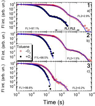
**Fig. 2** Normalized fluorescence decay transients of donor- $\sigma$ -acceptor compounds **1** (a), **2** (b) and **3** (c) in oxygensaturated (+O<sub>2</sub>) and oxygen-free (-O<sub>2</sub>) toluene solutions. Fractional intensities of initial and delayed fluorescence in -O<sub>2</sub> conditions are also noted.
