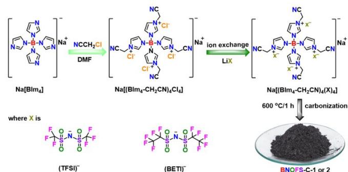
Fig. 1 Structures of the TSIL precursors,  $\text{Na}[(\text{BIm}_4\text{-CH}_2\text{CN})_4(\text{TFSI})_4]$  and  $\text{Na}[(\text{BIm}_4\text{-CH}_2\text{CN})_4(\text{BETI})_4]$ , and synthetic procedure for the production of multi-heteroatom-doped carbonaceous materials, BNOFS-C-1 and BNOFS-C-2.
