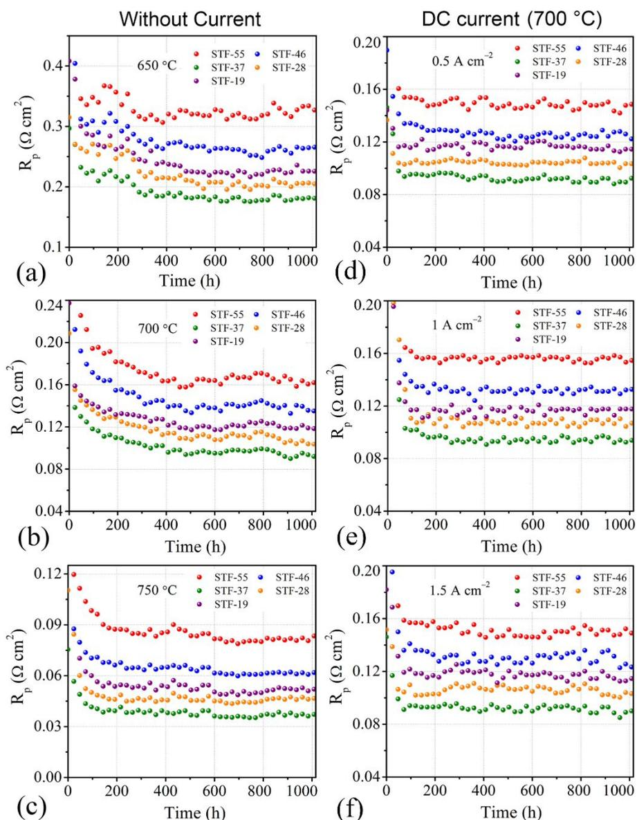
Fig. 6 Evolution of cell polarization resistance ( $R_p$ ) at 700 °C for the symmetric cells with STF electrodes; (a), (b), and (c) at different temperatures without current: (a) 650 °C, (b) 700 °C, (c) 750 °C; (e), (d), and (f) tested under 700 °C at different current densities: (e) 0.5 A cm<sup>-2</sup>, (d) 1.0 A cm<sup>-2</sup>, and (f) 1.5 A cm<sup>-2</sup>.
