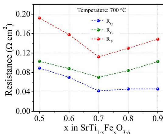
Fig. 9. G and  $R_Q$  values for different STF at 700 °C from the EIS fitting shown in Fig. S6.
