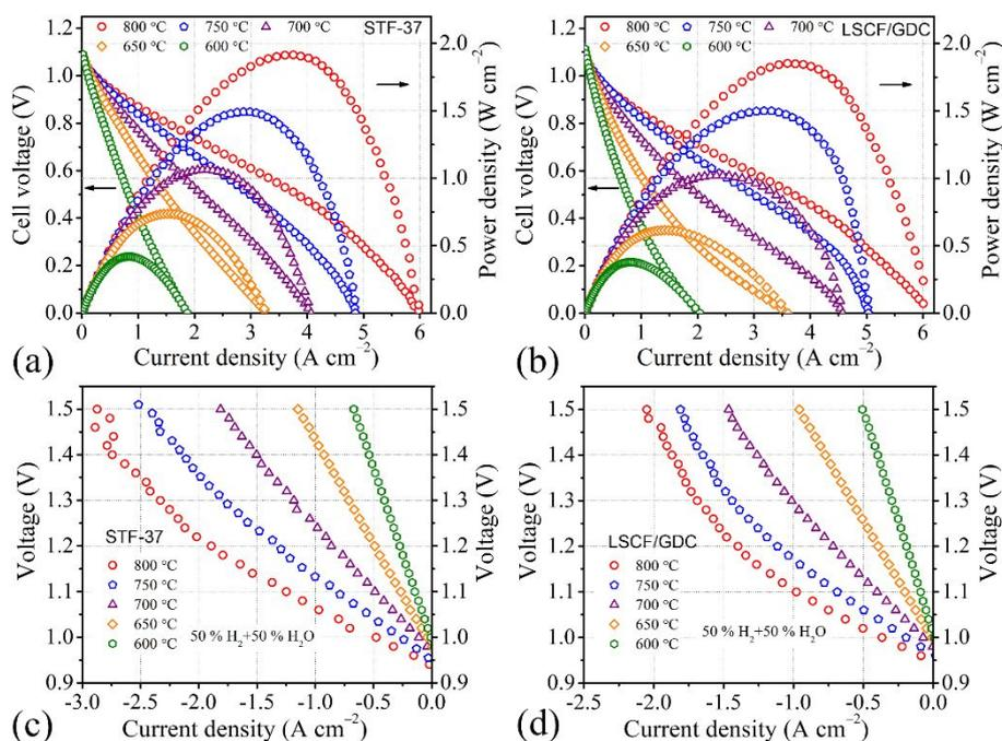
Fig. 8 Voltage and power density versus current density for a full cell with STF-37 (a) and LSCF/GDC (b) electrode measured at different temperatures in air and 3% H<sub>2</sub>O humidified hydrogen. Voltage versus current density for a full cell with STF-37 (c) and LSCF/GDC (d) electrode measured at different temperatures in air and 50 vol% H<sub>2</sub> + 50 vol% H<sub>2</sub>O.
