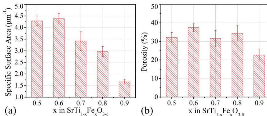
Fig. 3. Electrode specific surface area (a) and porosity (b) from the 2D image analysis for different STF electrodes.
