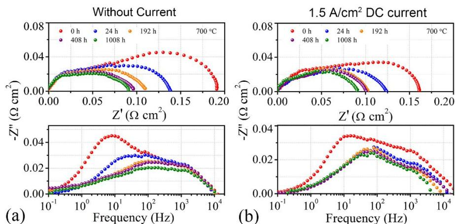
Fig. 5 Evolution of Typical Nyquist and Bode plots of EIS data measured at 700 °C for the symmetric cells with STF-37 electrode. (a) Without current; (b) With 1.5 A cm<sup>-2</sup> DC current.
