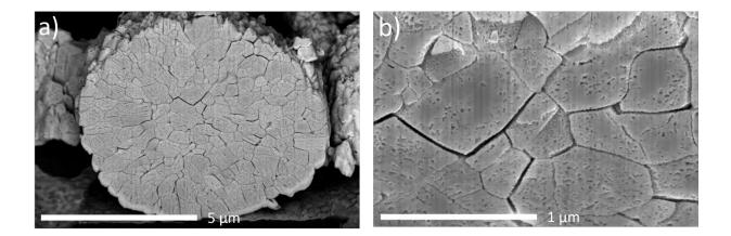
Figure 8: (a) Cross-sectional SEM image for a secondary NCA particle after focused ion-beam milling. Cross-section of particle indicates a homogenous distribution of mesopores within the particle core. (b) High magnification of the cross-section shown in (a).
