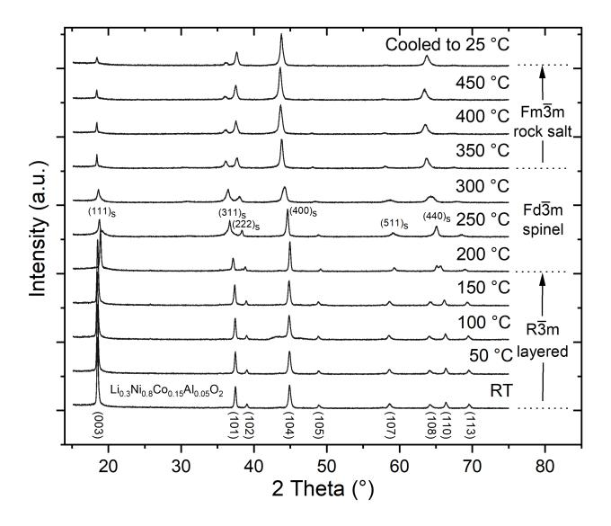
Figure 2: Temperature controlled XRD patterns of  $Li_{0.3}NCA$  powder upon heating to 450 °C.  $Li_{0.3}NCA$  powder was heated from 25 °C to 450 °C in 50 °C increments. At each increment, the temperature was held and XRD spectrum was collected. Visible peak ratio variations and shifts
