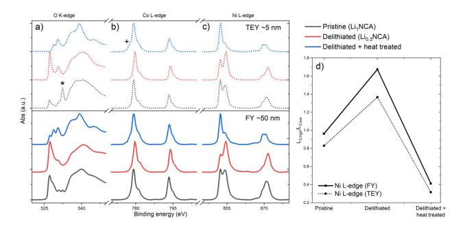
Figure 3: (a-c) Soft XAS O K-edge, Co L-edge and Ni L-edge spectra for pristine (Li<sub>1</sub>NCA), delithiated (Li<sub>0.3</sub>NCA), and delithiated + heat-treated NCA powders in TEY (5 nm) and FY (50 nm) modes. (d) Calculated Ni  $L_{3,high}/L_{3,low}$  ratios for all samples shown in TEY and FY mode. Peak marked with an asterisk in (a) is associated with Li<sub>2</sub>CO<sub>3</sub>. Plus sign in (b) is indicating slight reduction in Co.
