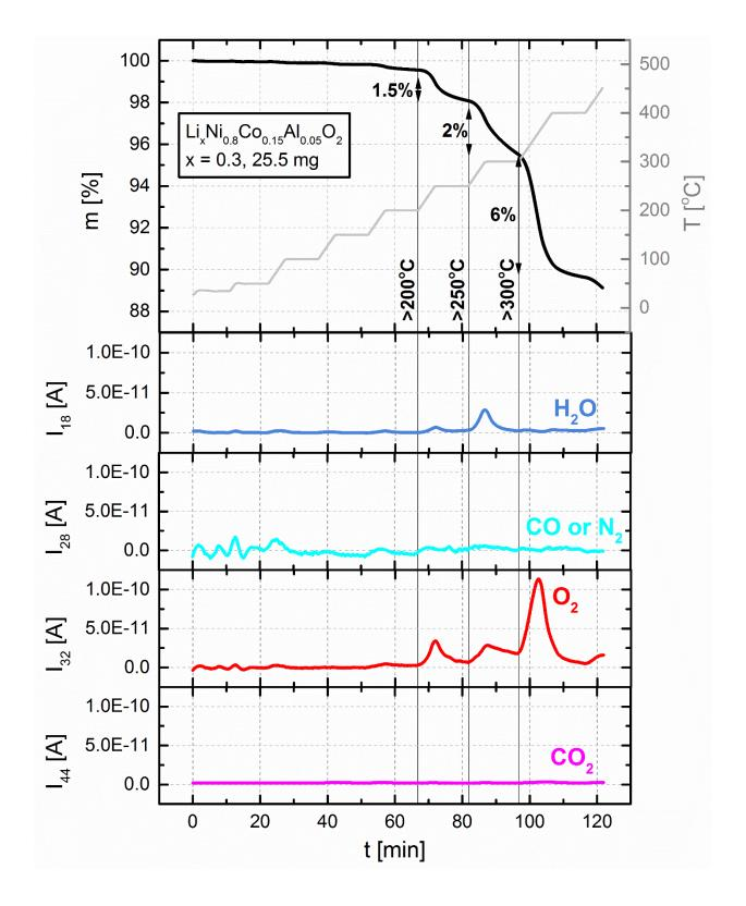
Figure 1: TGA-MS data of  $Li_{0.3}$ NCA powder. Delithiated samples were heated to 300 °C in 50 °C steps with a 10 °C/min rate (grey). Temperature was hold for 10 minutes at each step. After
