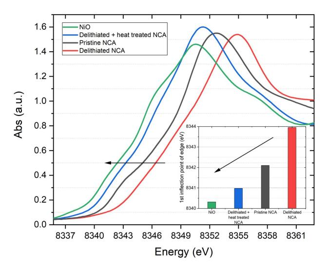
Figure 4: Normalized Ni K-edge XANES spectra of (black) delithiated Li<sub>0.3</sub>NCA, (blue) pristine NCA, (red) delithiated and heat-treated NCA, (green) NiO obtained in transmission mode. Retrieved data reflects the oxidation state of the bulk material. The edge position of NiO is used as a reference for Ni<sup>2+</sup>. The inset shows the edge energies derived from the 1<sup>st</sup> inflection point of the spectra.
