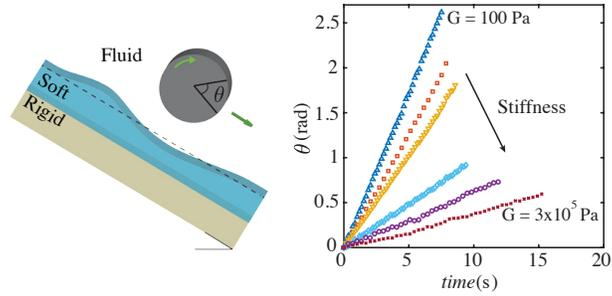
A fluid-immersed solid cylinder moves along a soft incline and rotates at a rate that depends on its aspect ratio and the stiffness of the incline.
