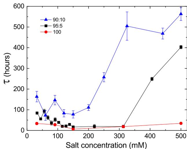
**Fig. 4** Delay time as a function of monovalent salt concentration, at different DLPE:DLPG ratios (mole %). At low salt concentrations ( $< 150$  mM), samples that contain DLPG (black and blue) show an increase in the delay time as salt concentration is decreased. At high salt concentrations ( $> 300$  mM) the opposite trend occurs. However, when the sample contains pure DLPE, there is no significant effect of the salt concentration on the delay time.
