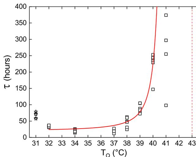
**Fig. 2** Delay time as a function of quenching temperature for pure DLPE. Empty squares represent measurements of individual capillaries at each quenching temperature. Solid red curve is the fit using Eq. (2), excluding the measurements at  $T_Q = 31$  °C (empty stars represent the  $L_\alpha \rightarrow L_\beta$  transition) and  $T_Q = 41$  °C due to the high variance caused by fluctuations. Red vertical dashed-line indicates the estimated  $T_{c \rightarrow \alpha}$  transition temperature.
