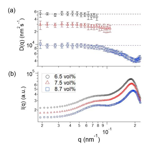
Fig. 6. (a) *q*-dependent diffusion coefficients D(q), obtained by dividing  $\Gamma$  by  $q^2$  for the short-term stationary samples with  $\phi_{HAp} = 6.5$ , 7.5, and 8.7 vol %. (b) Scattering intensity profiles obtained from the circularly averaged SAXS images for the samples with  $\phi_{HAp} = 6.5$ , 7.5, and 8.7 vol %.
