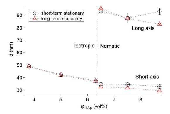
Fig. 2. Concentration dependence of the interparticle distance obtained from the SAXS measurements. The black circles and red triangles indicate the data for the short-term stationary (15 days after sealing) and long-term stationary (185 days after sealing) samples, respectively.
