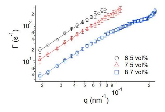
Fig. 5. *q* dependence of  $\Gamma$  obtained by fitting analysis using Eq. (2) for the short-term stationary samples with  $\phi_{\text{HAp}} = 6.5$ , 7.5, and 8.7 vol %. The solid lines represent the fitting lines proportional to  $q^2$  at q < 0.05 nm<sup>-1</sup>.
