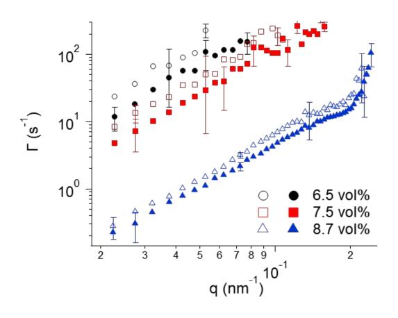
Fig. 8. *q* dependence of  $\Gamma$  obtained by fitting analysis using Eq. (3) for the long-term stationary samples with  $\phi_{\text{HAp}} = 6.5$ , 7.5, and 8.7 vol %. The open and closed symbols correspond to the  $\Gamma$  obtained from  $q_{//}$  and  $q_{\perp}$ , respectively. For clarity, only typical error bars are depicted.
