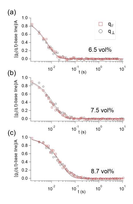
Fig. 4. Measured time autocorrelation functions  $g_2(q,t)$  at  $q = 3.76 \times 10^{-2}$  nm<sup>-1</sup> obtained from the XPCS measurements for the short-term stationary samples with  $\phi_{\text{HAp}} =$  (a) 6.5, (b) 7.5, and (c) 8.7 vol %. The red squares and black circles indicate the data for  $g_2(q_{//},t)$  and  $g_2(q_{\perp},t)$ , respectively. The solid lines represent the fitting curves obtained using Eq. (2).
