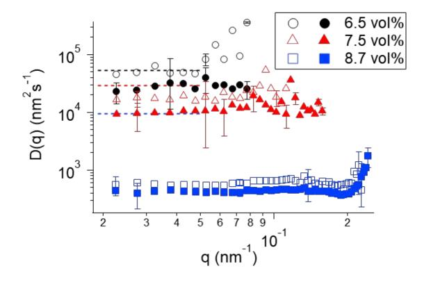
Fig. 9. Variation of D(q), obtained by dividing  $\Gamma$  by  $q^2$ , for the long-term stationary samples with  $\phi_{\text{HAp}} = 6.5$ , 7.5, and 8.7 vol %. The open and closed symbols correspond to the D(q) obtained from  $q_{//}$  and  $q_{\perp}$ , respectively. For clarity, only typical error bars are depicted. The dashed lines indicate the diffusion coefficients for the short-term stationary samples at q < 0.05 nm<sup>-1</sup>.
