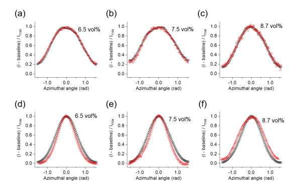
Fig. 3. Azimuthal scattering intensity profiles for the peak of I(q) obtained at (a)–(c) the low-q side and (d)–(f) the high-q side for the samples with  $\phi_{HAp} = 6.5$ , 7.5, and 8.7 vol %. The black circles and red triangles indicate the data for the short-term stationary and long-term stationary samples, respectively.
