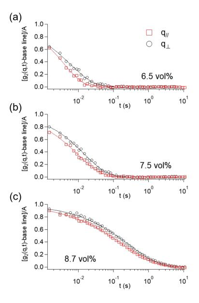
Fig. 7. Measured time autocorrelation functions  $g_2(q,t)$  at  $q = 4.76 \times 10^{-2}$  nm<sup>-1</sup> obtained from the XPCS measurements for the long-term stationary samples with  $\phi_{\text{HAp}} =$  (a) 6.5, (b) 7.5, and (c) 8.7 vol %. The red squares and black circles indicate the data for  $g_2(q_{//},t)$  and  $g_2(q_{\perp},t)$ , respectively. The solid lines represent the fitting curves obtained using Eq. (3).
